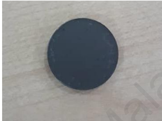
Figure 3.1: Compacted and sintered final Al/GNP tablet (same for all three GNP compositions)
