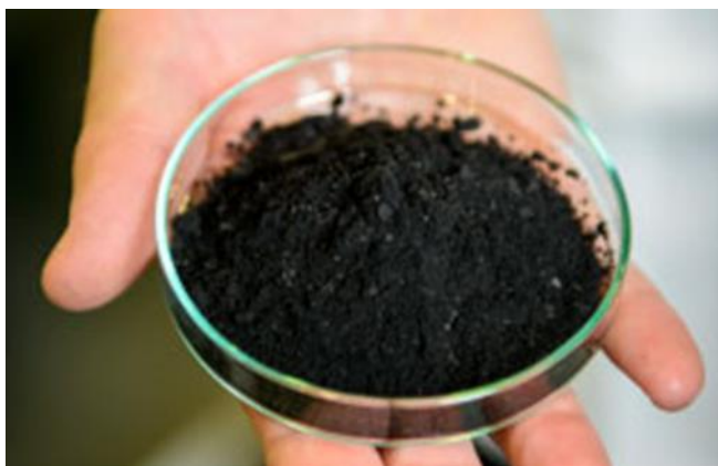
Figure 2.6: Graphene nanoplatelets aggregate (Kumar P., 2014)
