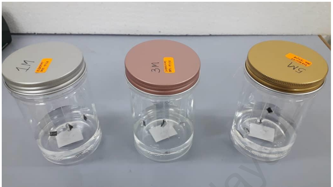
Figure 3.4: Immersing the test samples in NaCl solutions of 1M, 3M and 5M
