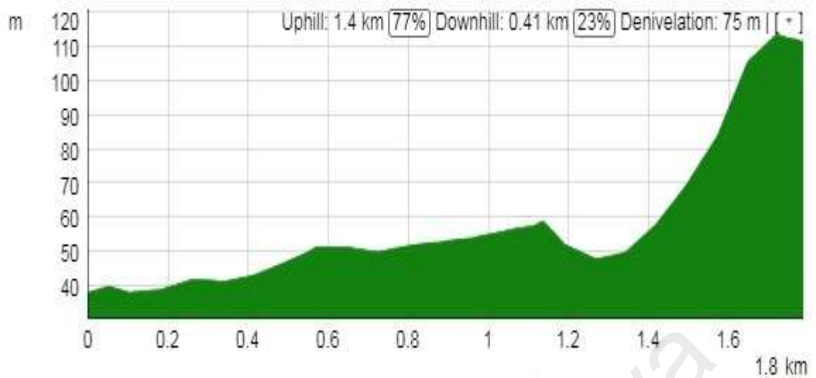
Figure 3.4: Piping profile from power station to reservoir
