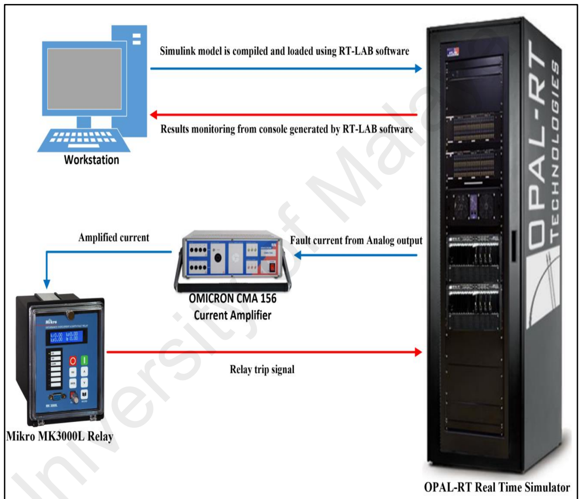
Figure 3.20: Block diagram of relay testing using Opal-RT real-time simulator.
