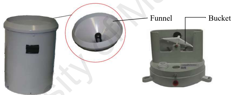
Figure 2.16: Tipping Bucket TB3 Model
