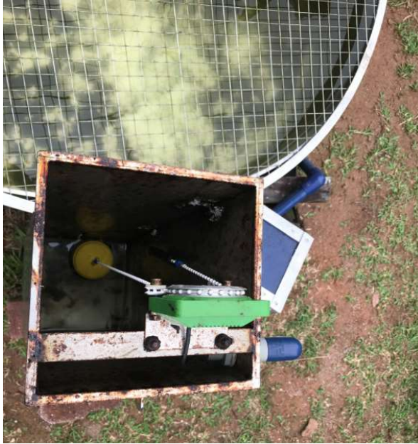
Figure 3.10: Corroded pan at different angle
