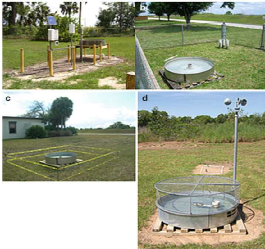
Figure 2.2: Various setups of US class A evaporation pan (Abtew & Malesse, 2013)
