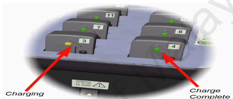
Figure 3.5: Sensor LED feedback for battery charging status (DELSYS Incorporated, 2018).
