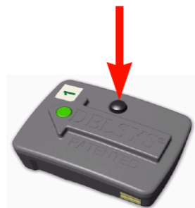
Figure 3.7: Turning the TRIGNO™ Sensor "ON" (DELSYS Incorporated, 2018).
