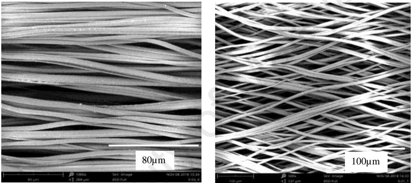
Figure 4.1 FESEM images of Polyurethane scaffolds (a) Scaffold with parallel 0% HA 1000x magnification (b) Scaffold with non-parallel fibers and 1% HA 500x magnification
