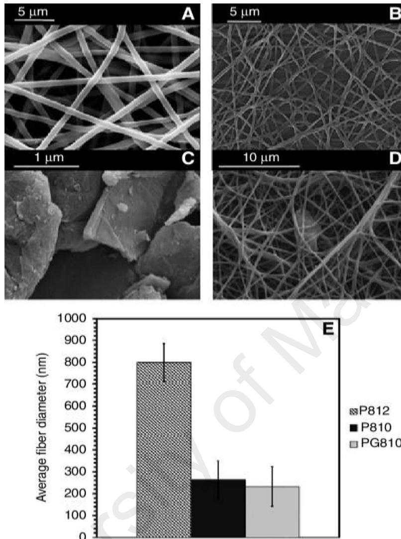
Figure 2.3 Scanning Electron Microscopy graphs (A-D) and mean fiber diameter (E) of electrospun polyurethane scaffolds (Safikhani, Zamanian et al. 2017)
