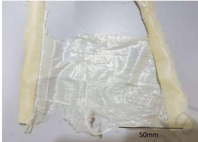
Figure 3.5 Picture of the polyurethane scaffold with parallel aligned fibers, no HA added
