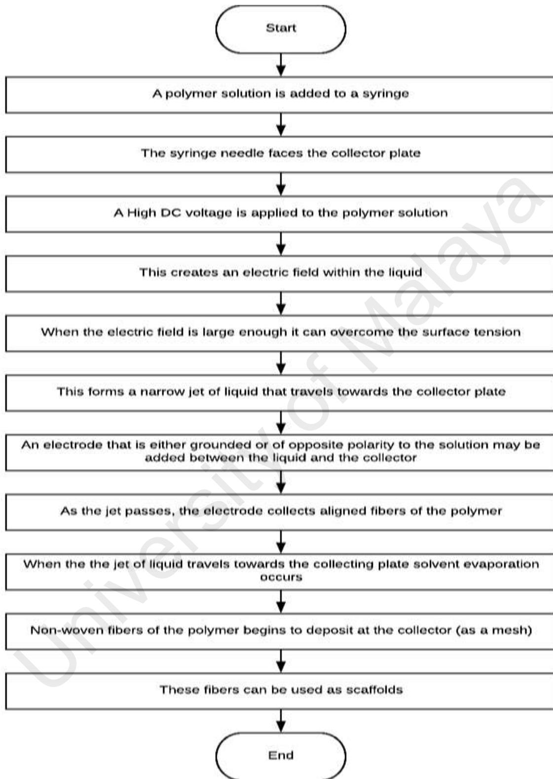
Figure 2.1 Flowchart explaining the process of electrospinning
