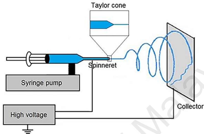
Figure 2.2 This diagram illustrates the process of electrospinning and the required components for the nano-fibers to form (Zhao, Shi et al. 2011).
