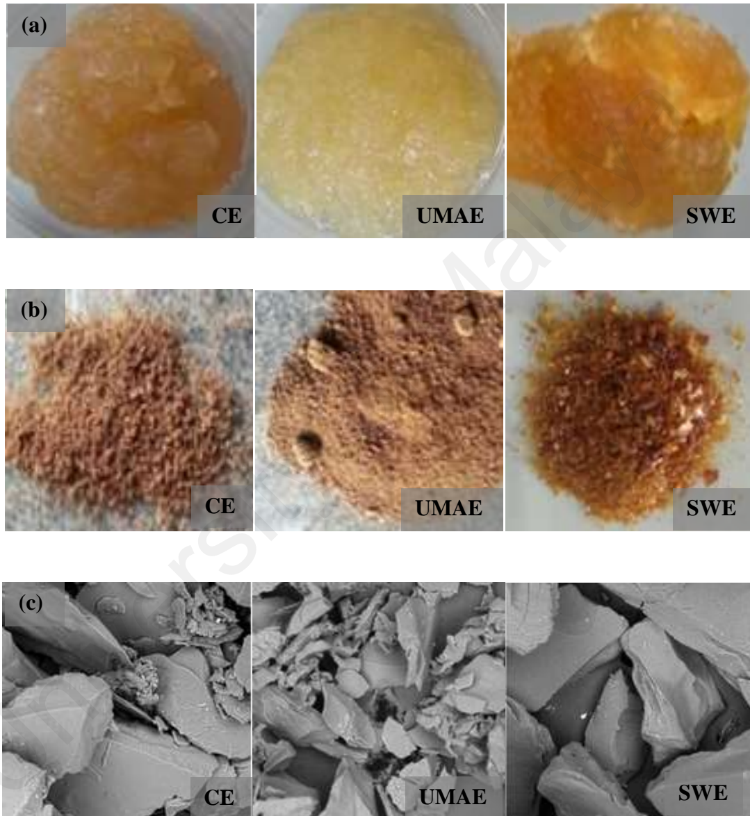
Figure 4.17: Photographs of (a) wet pectin, (b) dried pectin and (c) scanning electron micrograph of pectin from CE, UMAE and SWE; at 500× magnification, 100µm.
