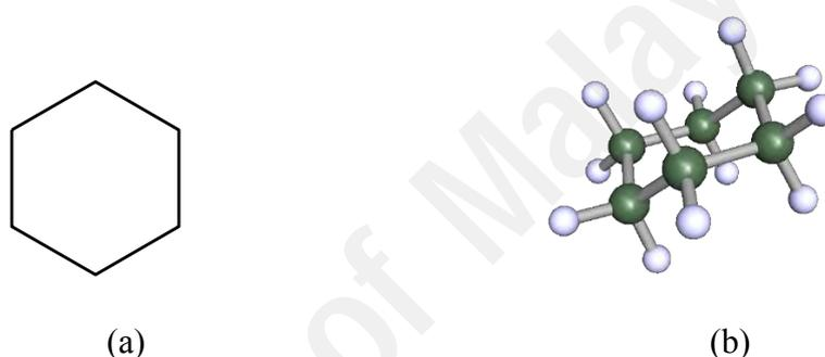
**Figure 2.3: Structure of cyclohexane in view of (a) a flat hexagon and (b) the most-stable chair conformation**
