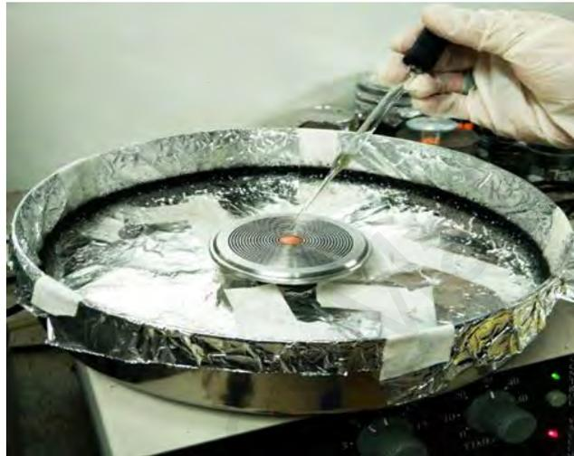
**Figure 3.17 :  $\text{Bi}_2\text{Se}_3$  composite onto a cuprum plate by the spin-coating method**
