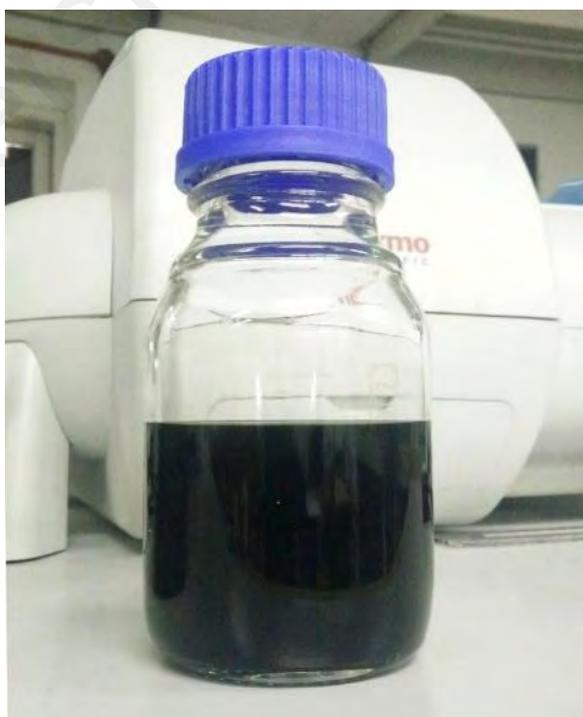
**Figure 3.3: The graphene suspension after the electrochemical process.**
