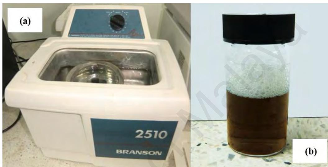
**Figure 3.10 : Preparation of the GO composite solution (a) Mixing of GO solution with the PEO host polymer using an ultrasonic bath (b) the mixed suspension GO polymer solution**
