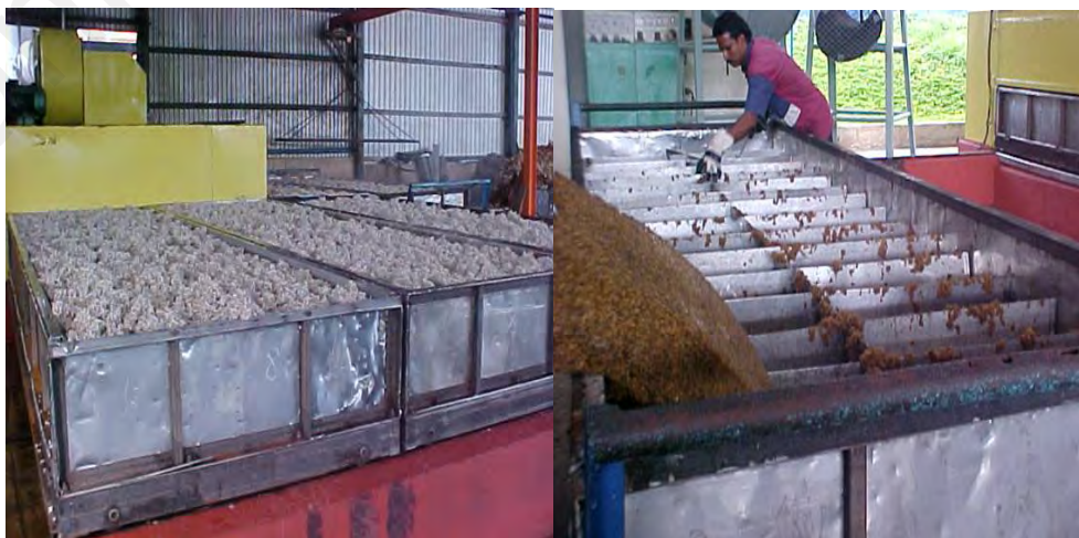
Figure 3.25: Wet rubber crumbs are transformed into dried rubber after drying
