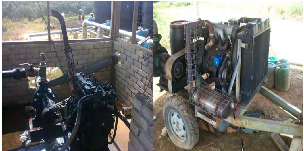
Figure 3.9: Diesel engine used to run the water sprinkler system.
