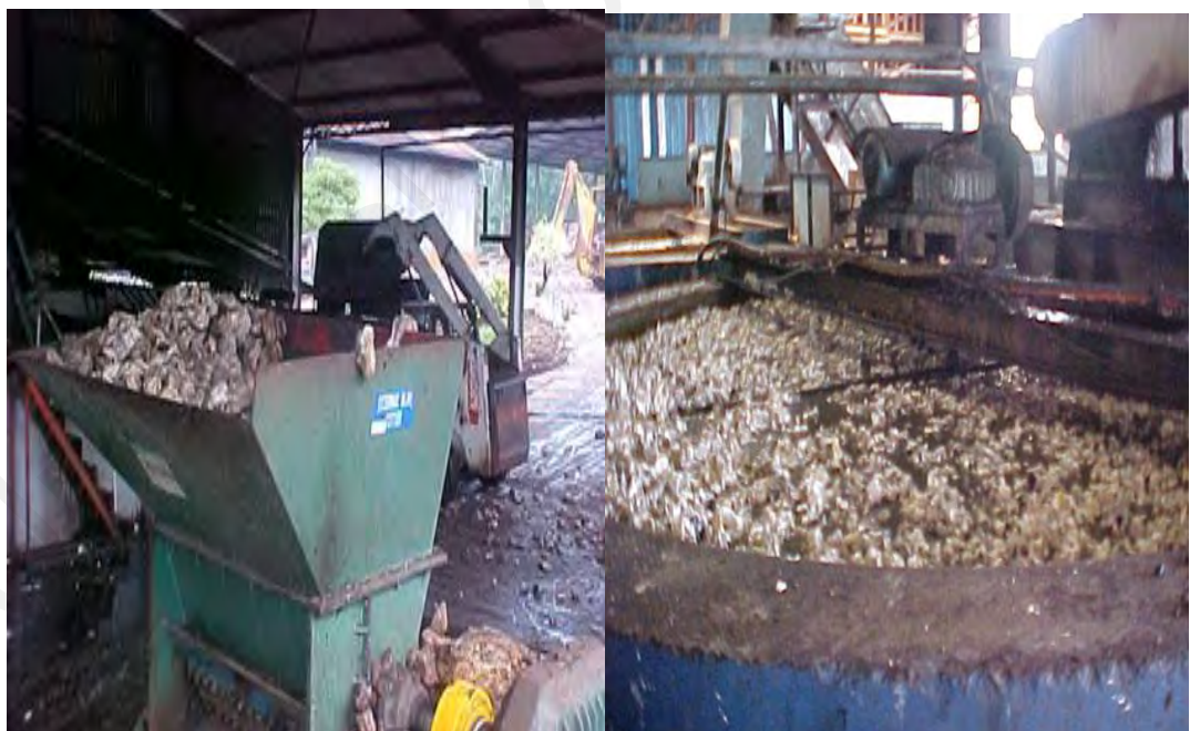
Figure 3.22: Pre-cleaning and size reduction process (Source: Tan,MRB).
