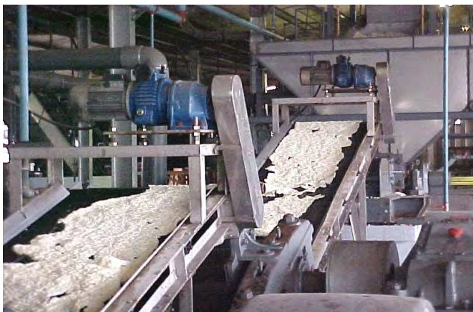
Figure 4.39: A typical creping section in the production of SMR block rubber
