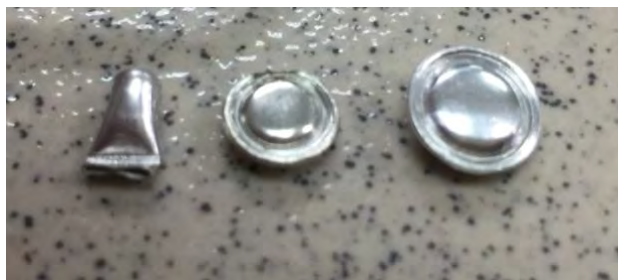
Figure 5.3: Hermetically sealed pans containing liquid samples: Tin cylinder (left), Tin pan (middle) and Aluminum pan (right)
