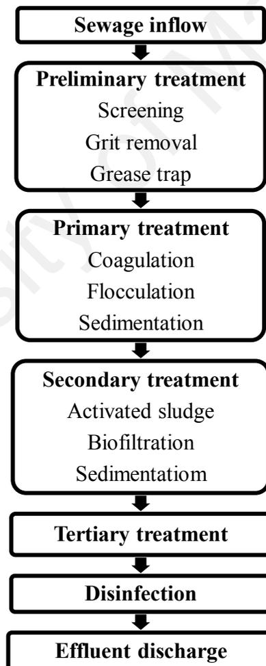
**Figure 2.2:** Flow diagram for wastewater treatment plants (WWTP).
