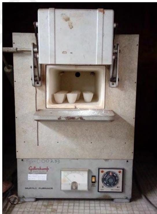
Figure 3.11: Furnace used for loss on ignition (LOI) analysis.
