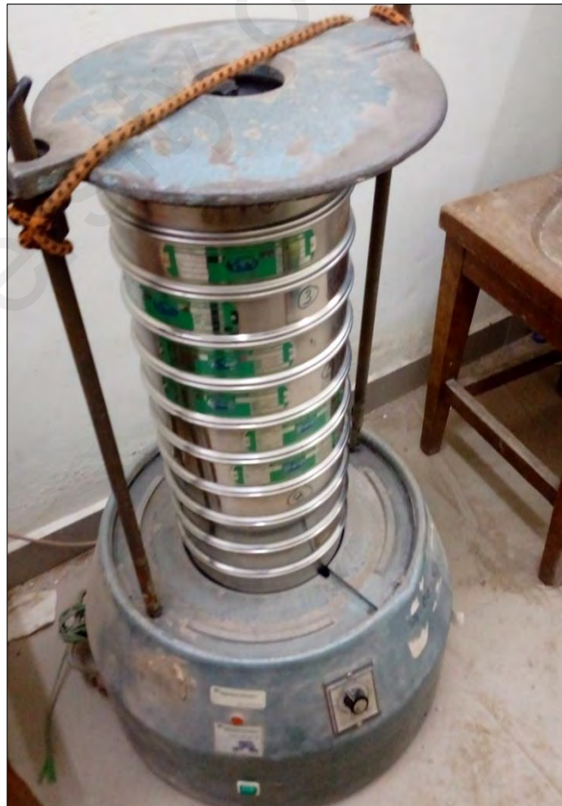
Figure 3.9: Test sieves and mechanical sieve shaker.
