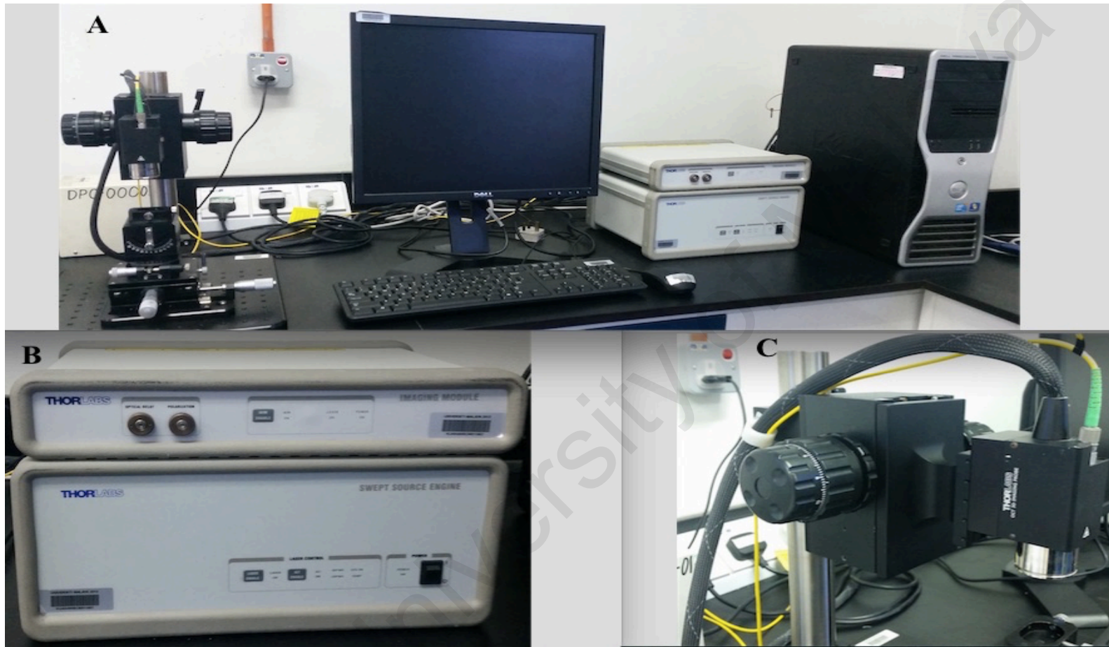
Figure 3.4: Photograph of (A) THORLABS CS1300SS OCT Imaging System (USA) Components. (B) Thorlabs OCS 1300 SS engine and imaging module. (C) Probe and stand.
