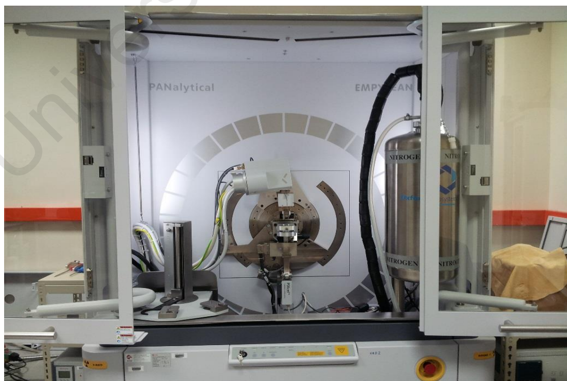
Figure 3.4: The SAXS instrument used for size characterisation of AgNPs.
