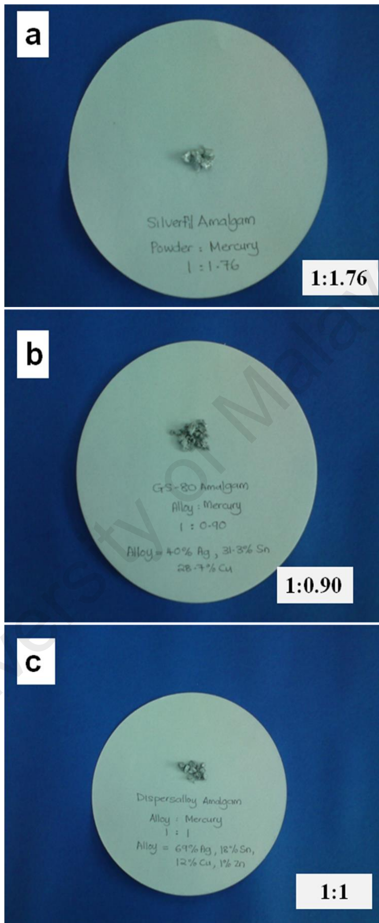
Figure 4.30: Physical appearances of the triturated amalgams. a) Silverfil™, b) GS80, and c) Dispersalloy.
