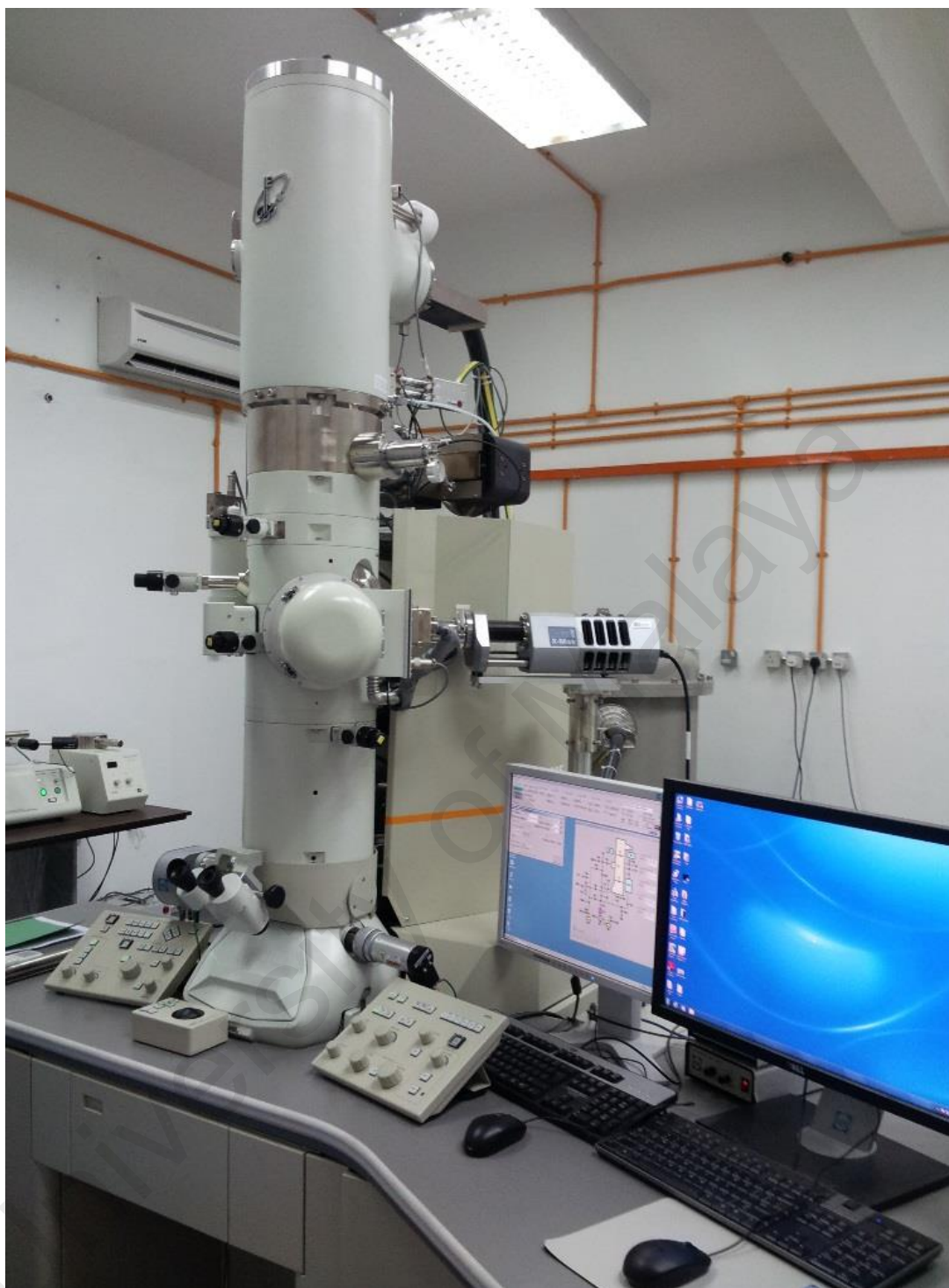
Figure 3.5: The HRTEM instrument used for morphological investigation of AgNPs.
