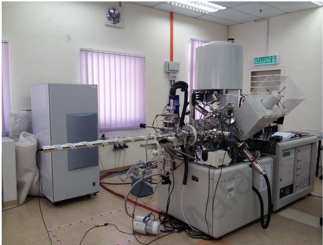
Figure 3.1: The XPS equipment used for chemical analyses of Silverfil™ starting materials as well as the varied set amalgams.
