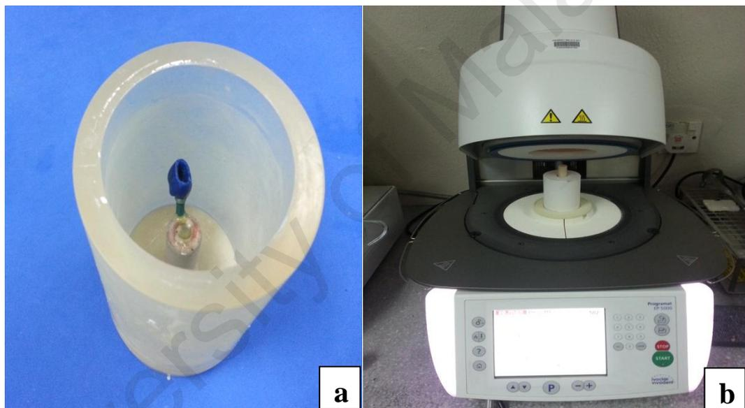
**Figure 3.11:** a) Spruing the wax pattern into the investment mould, b) Heat pressing of IPS e.Max Press ingot
