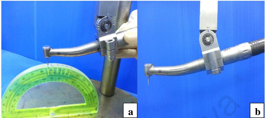
**Figure 3.5:** a) The jig used for setting the tapered angle, b) The jig used for fixation the handpiece at the oriented angle
