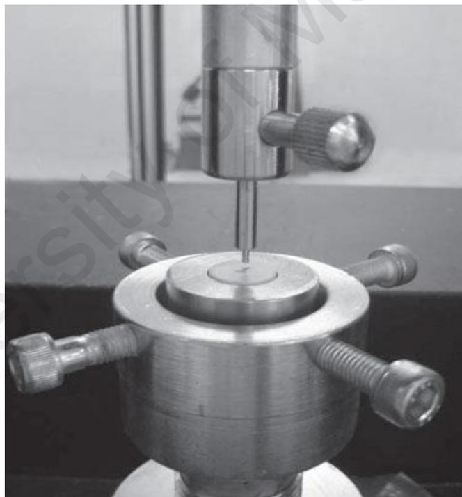
**Figure 2.4:** Biaxial flexural strength test, Adopted from (Al-Makramani et al., 2010)
