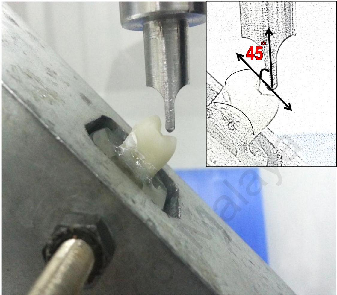
**Figure 3.18:** Specimen during the test (oblique loading)
