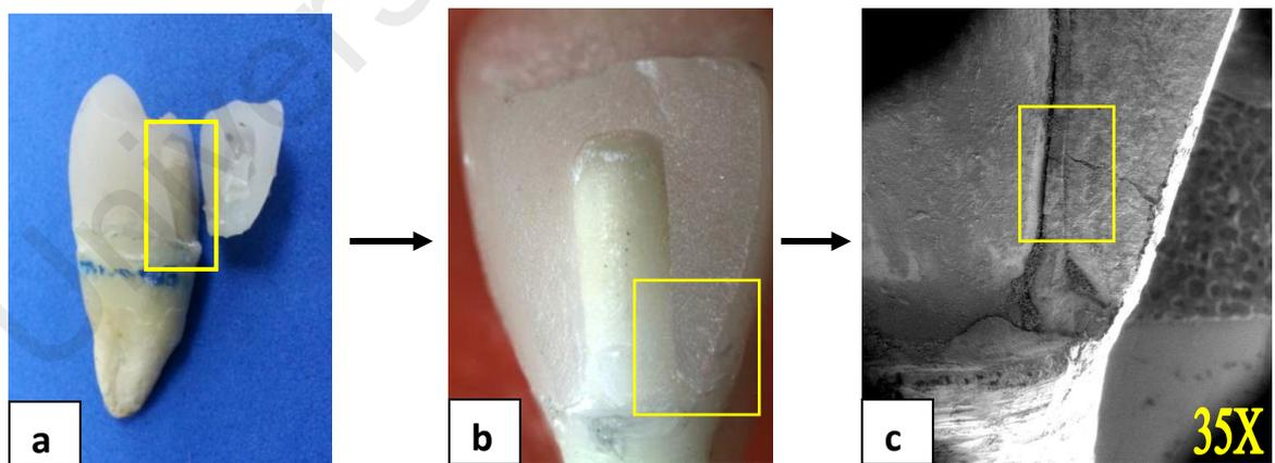
**Figure 4.8:** Optical (a,b) and SEM (c) images of fractured CEREC specimen; proximal (a) and palatal (b,c) view
