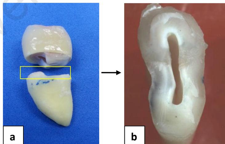
**Figure 4.14:** Optical images of fractured tooth in Cercon group; proximal (a) and cross-sectional (b) view
