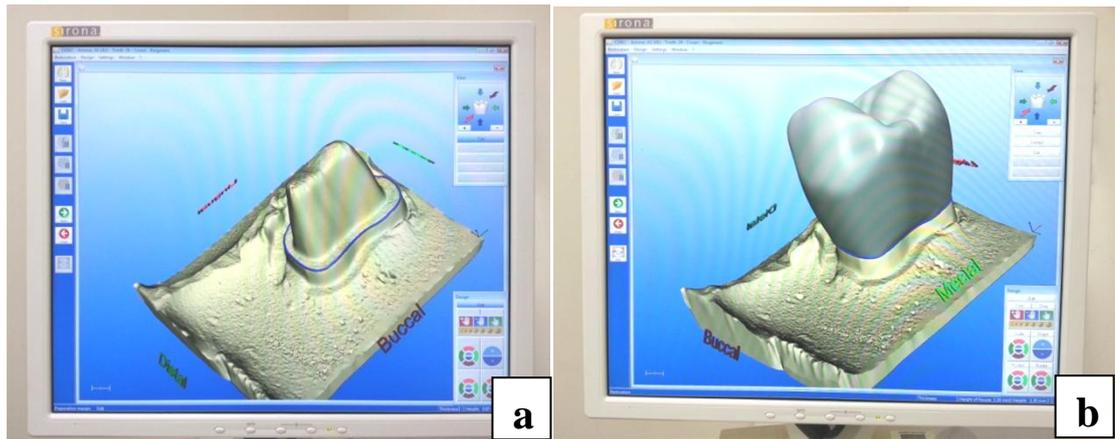
**Figure 3.8:** CEREC acquisition unit; a) Optical impression, b) Crown designing
