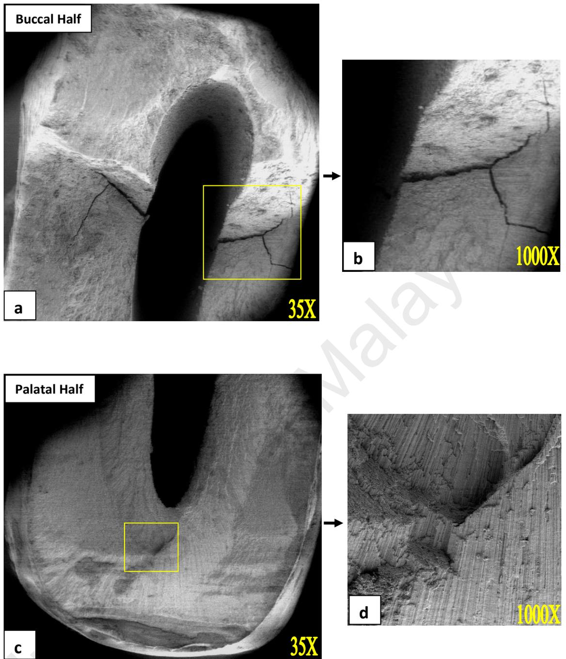
**Figure 4.15:** Cross-sectional SEM view of fractured tooth surface in Cercon group
