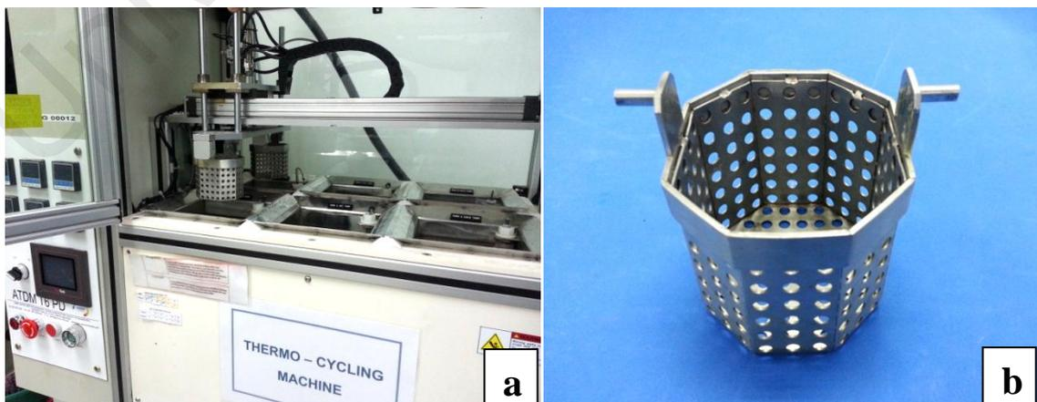
**Figure 3.16:** a) Thermocycling machine, b) Specimens holder (mesh)
