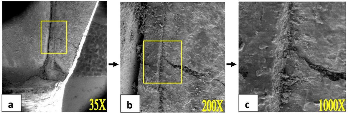
**Figure 4.9:** SEM micrographs of fractured CEREC specimen at different magnifications
