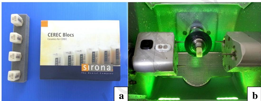
**Figure 3.9:** Milling Process; a) CEREC blocks, b) CEREC milling machine
