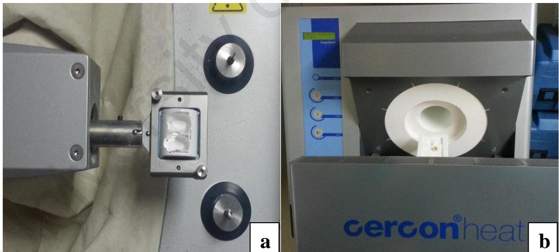
**Figure 3.13:** a) Cercon coping milling, b) Coping sintering
