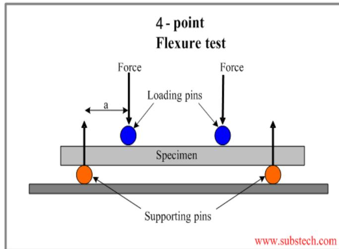
**Figure 2.2:** Four-point bending test, Adopted from (www.substech.com)
