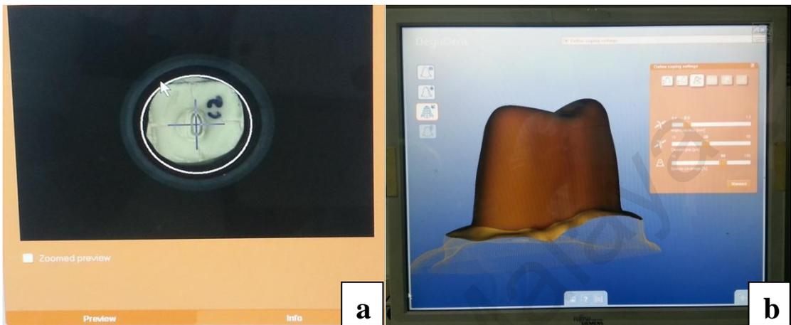
**Figure 3.12:** a) Die scanning in Cercon eye, b) Coping designing
