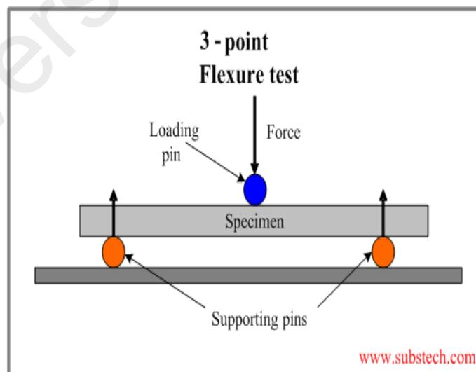
**Figure 2.3:** Three-point bending test, Adopted from (www.substech.com)
