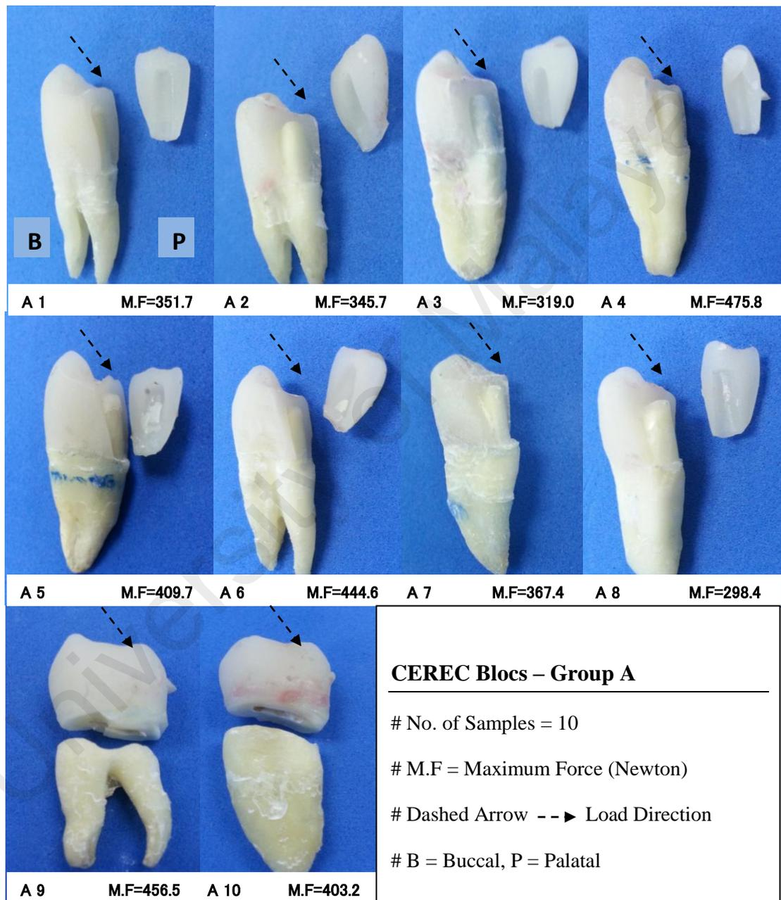
**Figure 4.5:** Failure patterns of CEREC Blocs specimens; ceramic crown fracture (A 1 to A 8) and severe tooth fracture (A 9 and A 10)
