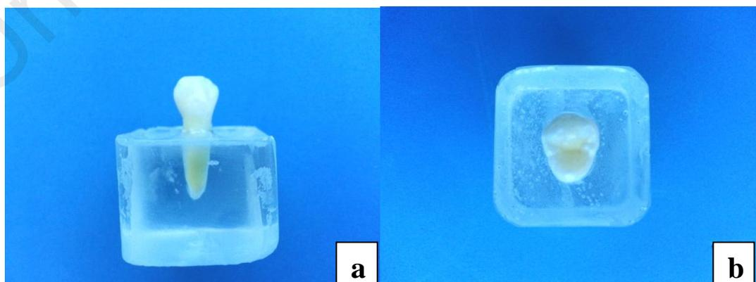
**Figure 3.3:** The tooth mounted in the epoxy resin; a) Buccal view, b) Occlusal view
