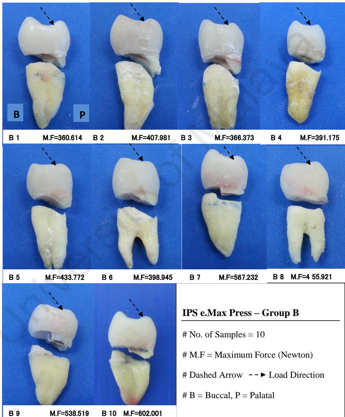
**Figure 4.6:** Failure pattern of IPS e.Max Press specimens (Severe tooth fracture)
