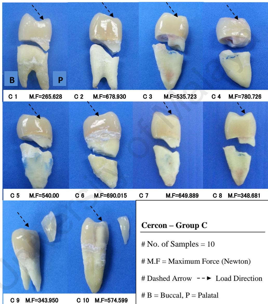
**Figure 4.7:** Failure patterns of Cercon; Severe tooth fracture (C 1 to C 8) and ceramic crown fracture (C 9 and C 10)
