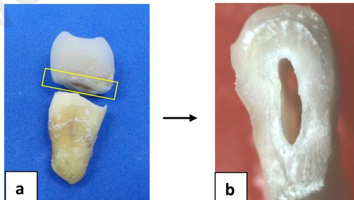
**Figure 4.11:** Optical images of fractured tooth in IPS e.Max Press group; proximal (a) and cross-sectional (b) view
