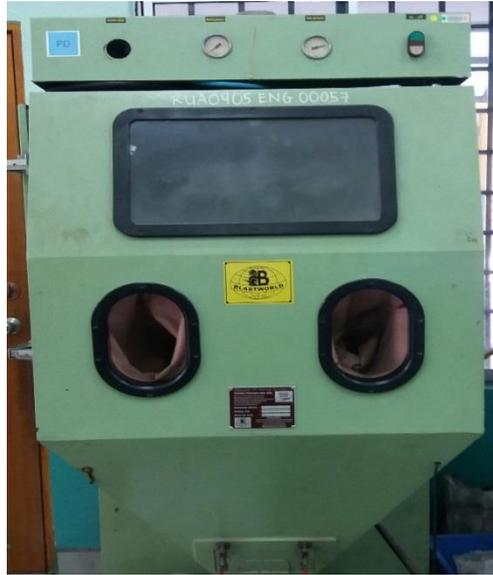
Figure 3: Shows the sandblasting machine (SB-8060-KP Techno Finishing Sdn. Bhd. Malaysia.) used for this study.
