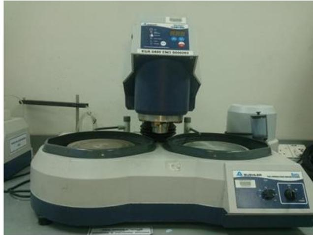
*Figure 2:* Twin variable grinding and polishing machine (250 High Speed Twin Grinder-Polisher by Buehler) was used for gritting the CPTi surfaces.
