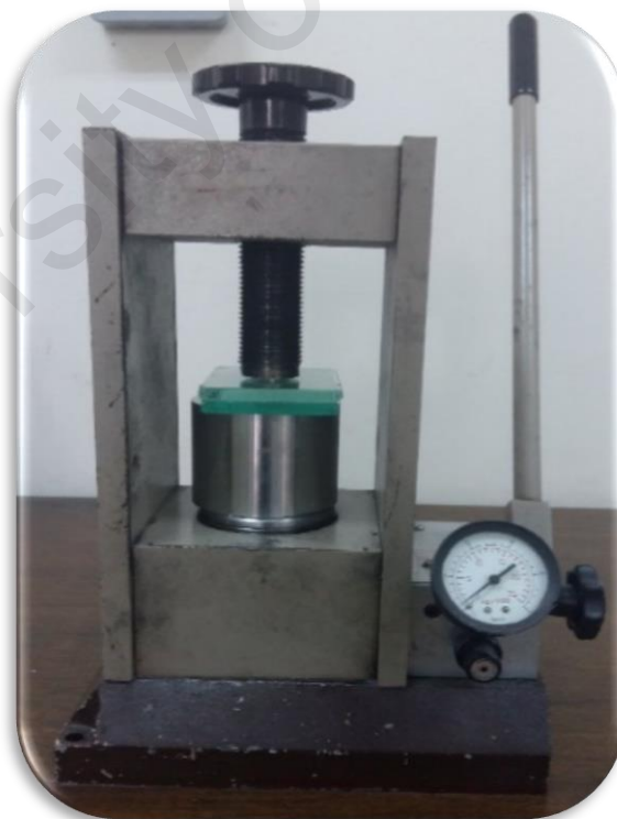
Figure 3.18: Uni axial hydraulic used to apply 150N.
