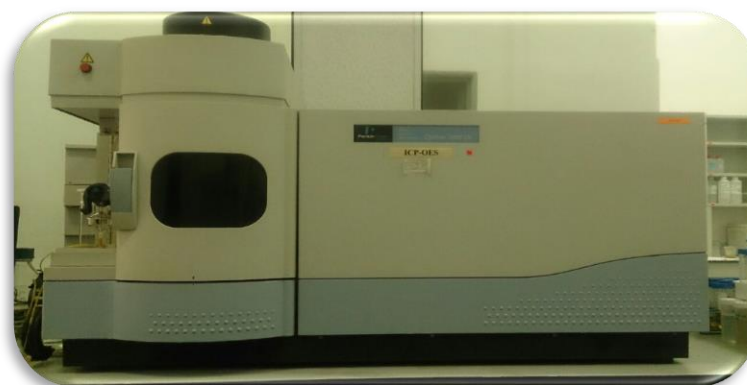
Figure 3.14: ICP-OES – for metal analysis.
