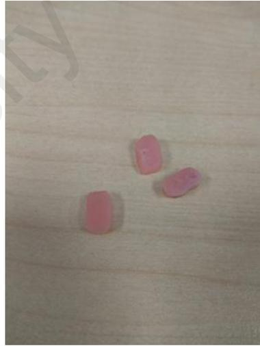
**Figure 3-7: Cylindrical samples prepared for cytotoxicity test**
