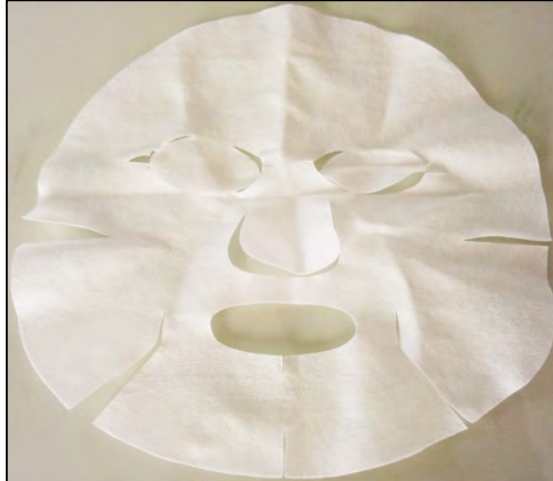
Figure 3.5: The disposable cotton mask sheet that used to connect the coupling devices of the working electrode and the human skin
