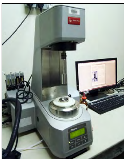
Figure 3.2: Physica MCR 301 Rheometer that used for viscosity measurement of the topical viscous hydrocolloid solution
