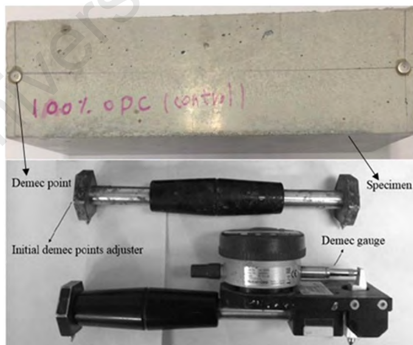
Figure 3.5: Drying shrinkage measurement
