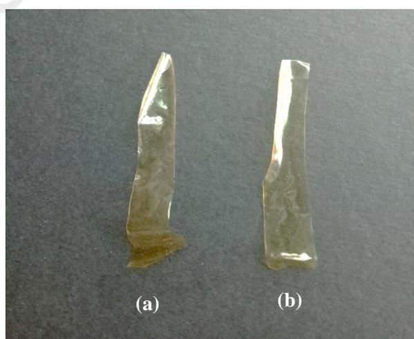
**Figure 4.15: Tensile test samples at wet states, a) Ch-g-PVA b) BSA/Ch-g-PVA.**
