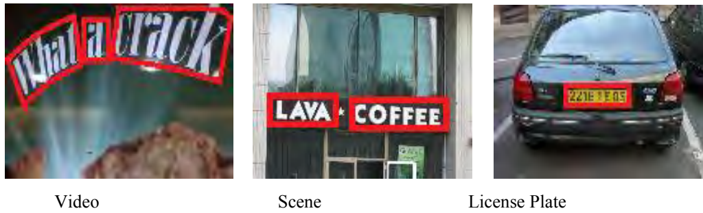
Figure 5.21: Sample word detection results of the proposed approach for different databases.
