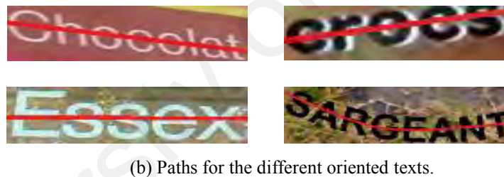
Figure 7.7: Examples of path estimation for the arbitrary oriented text using fused results with angles.
