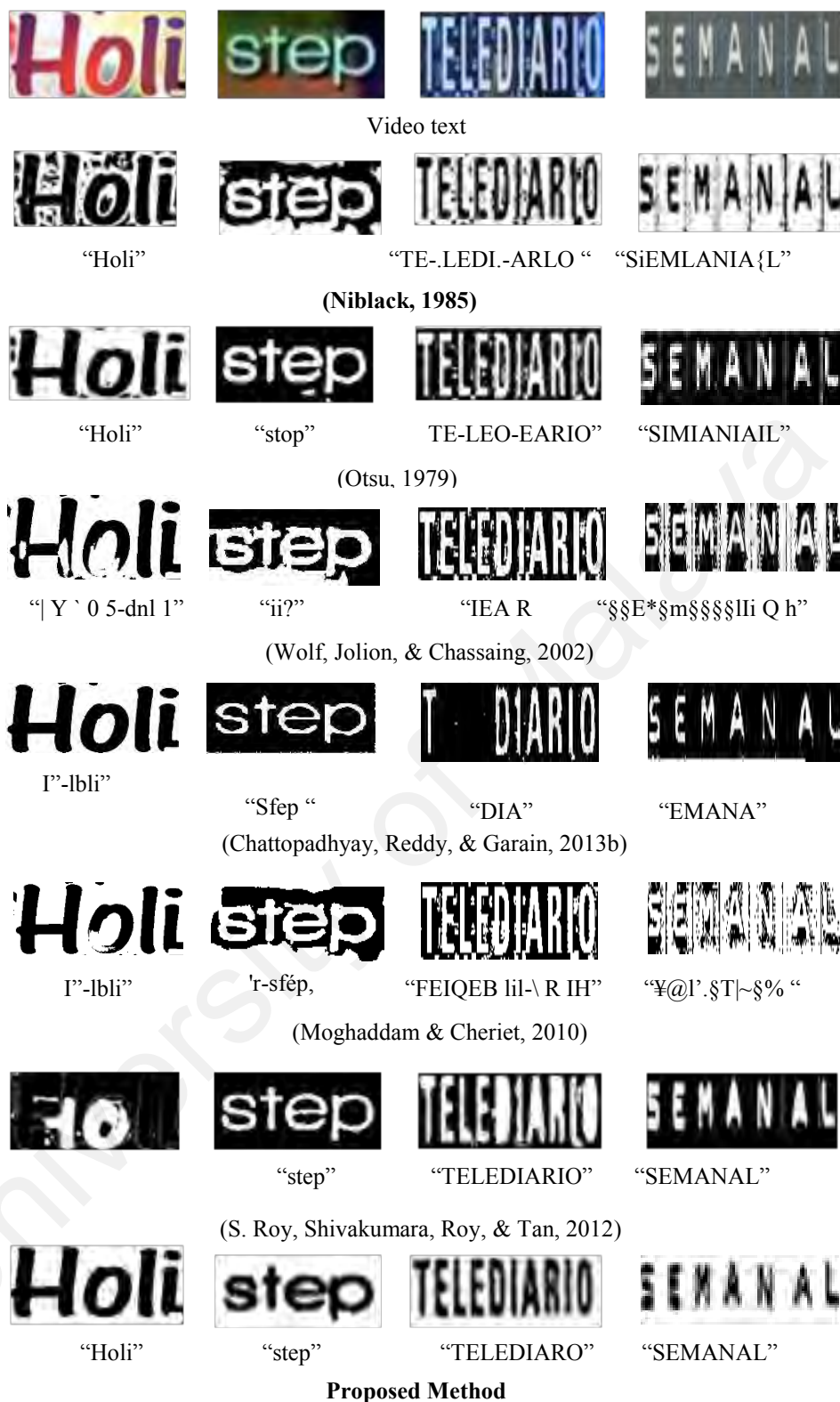
Figure 7.9: Binarization and recognition results of the proposed and existing methods on collected data and Hua’s data.
