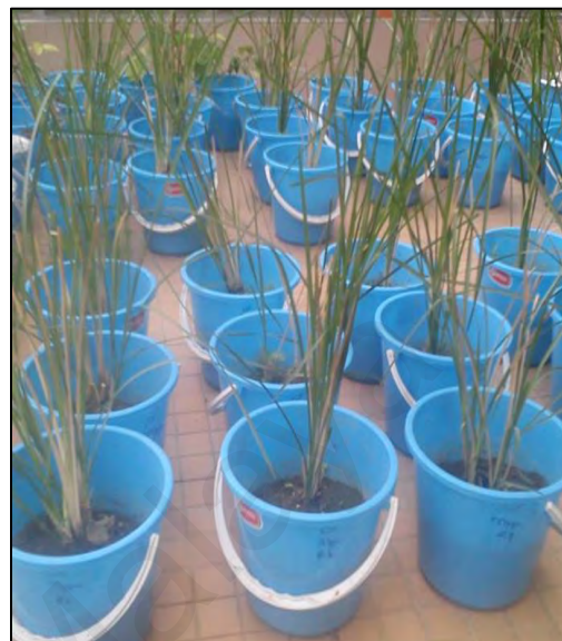
Figure 11.6: Undergoing experiment using different types of low cost soil amendments with Vetiver grass (Chapter 6)
