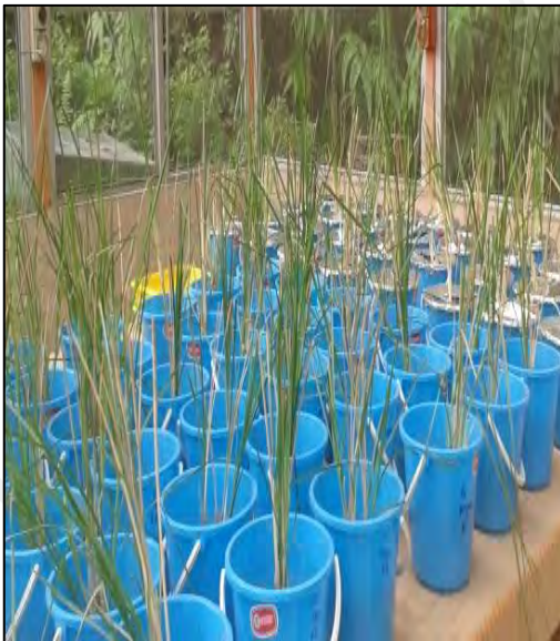
Figure 10.3: Undergoing Cd and Pb phytotolerance experiment with Vetiver grass (Chapter 4)
