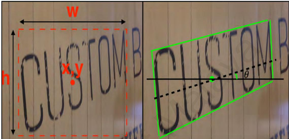
**Figure 2.10:** In comparison to the encoding of axis-aligned bounding box on the left ( $x, y, w, h$ ), rotational bounding box has an extra bit of information,  $\theta$ , which is the angle offset between the text line and the horizontal axis.
