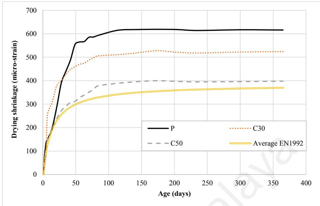
**Figure 8.2: Development of drying shrinkage (Experimental and average EN1992 (2010) prediction)**
