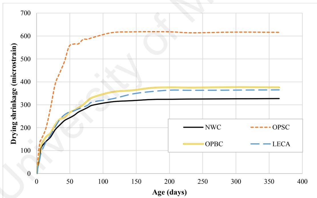
**Figure 7.5: Development of drying shrinkage strains under 7-days moist curing**
