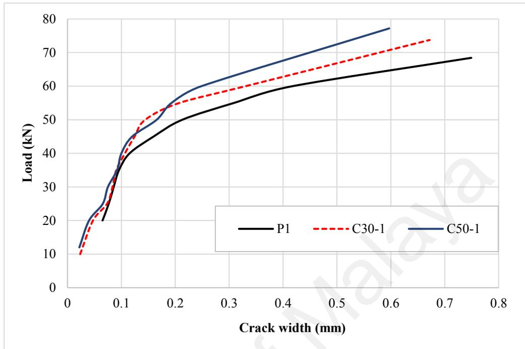
**Figure 9.11: Development of cracks widths of Grade 25 concrete beams**
