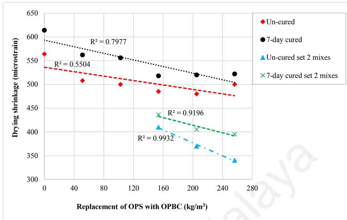
**Figure 6.9: 234-days age shrinkage versus the replacement of OPS by OPBC aggregates**
