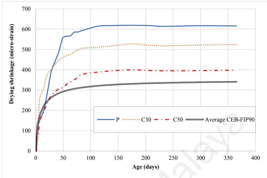
**Figure 8.4: Development of drying shrinkage (Experimental and average CEB/FIP90 (2001) prediction)**
