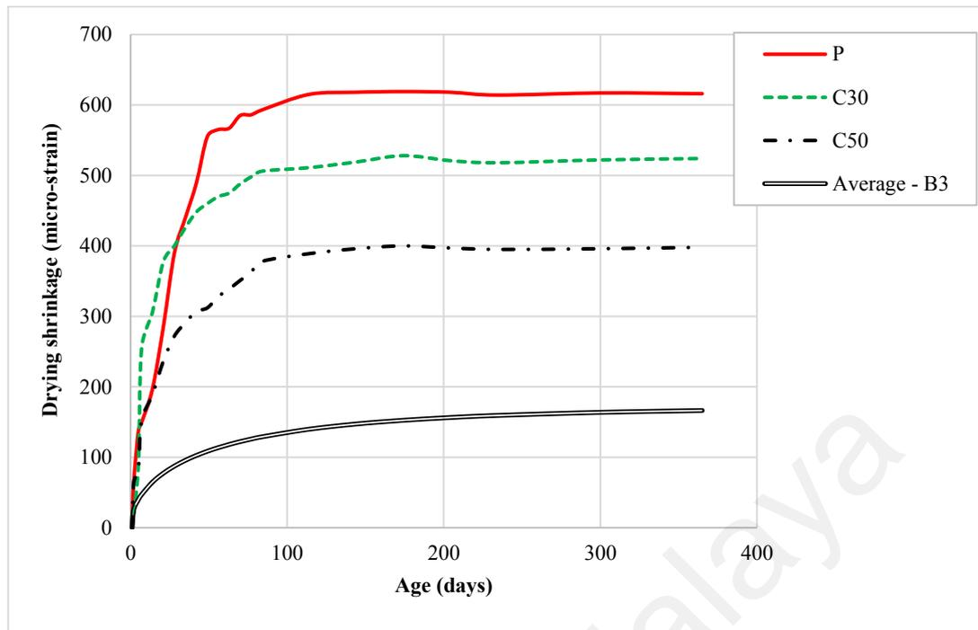
**Figure 8.10: Development of drying shrinkage (Experimental and average B3 model predictions)**
