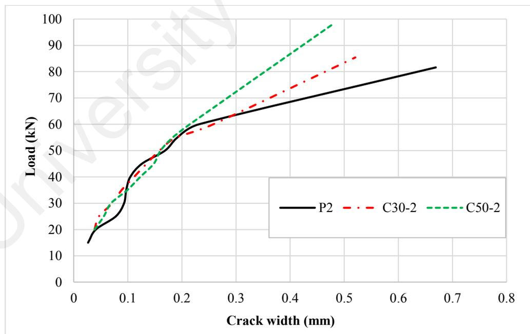
**Figure 9.12: Development of cracks widths of Grade 35 concrete beams**
