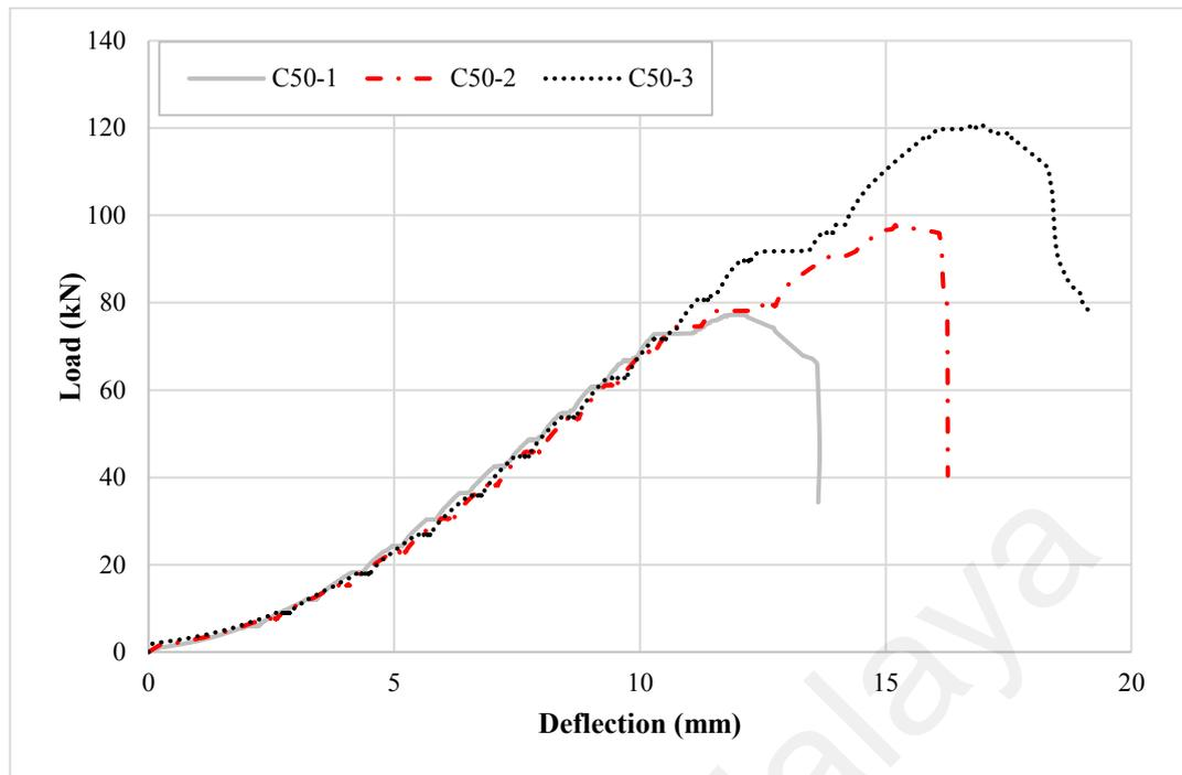
**Figure 9.5: Structural behaviour of OPS-OPBC50% concrete beams (set-3) without shear reinforcement**
