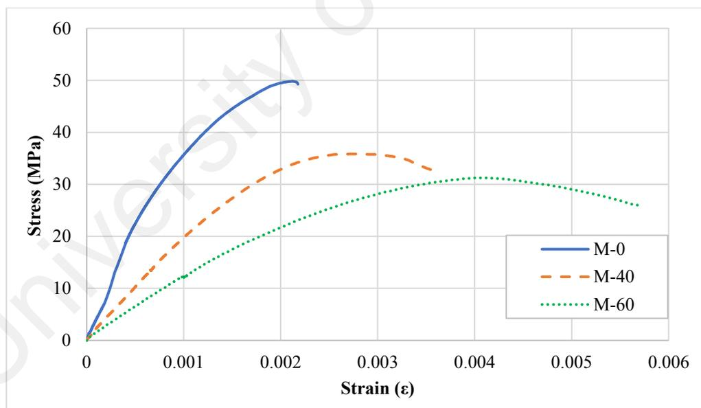
**Figure 5.6: Stress-strain curves for the prepared concrete mixes**
