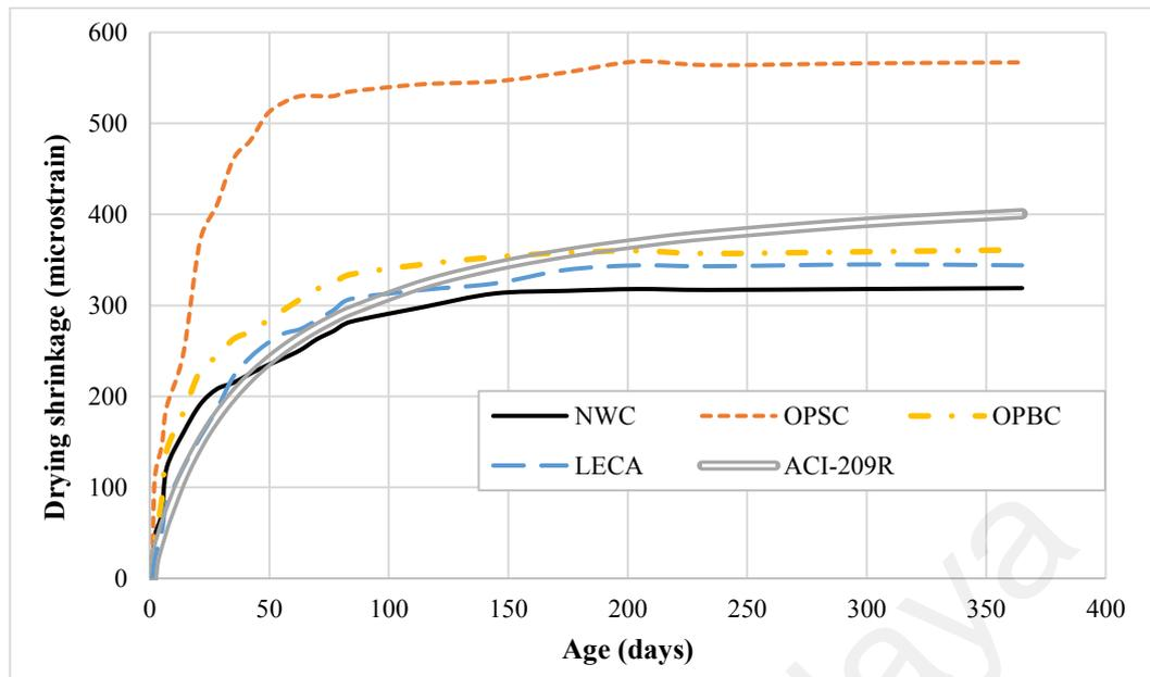
**Figure 7.6: Development of drying shrinkage with average prediction model results under air-drying condition**
