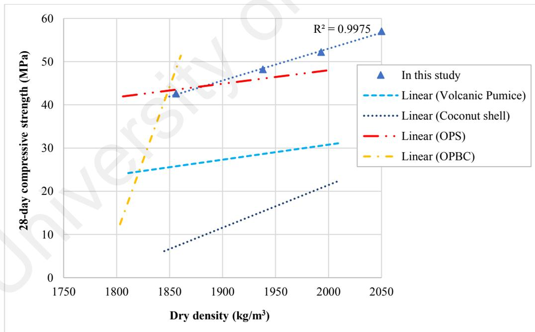
**Figure 5.2: The relationship between the dry density and 28-day compressive strength of OPBC-OPS mixes and comparison with OPS concretes (OPSC); palm oil clinker concrete containing OPBC as coarse and fine; high strength lightweight concrete containing scoria aggregate; volcanic pumice lightweight concrete and coconut shell concretes**
