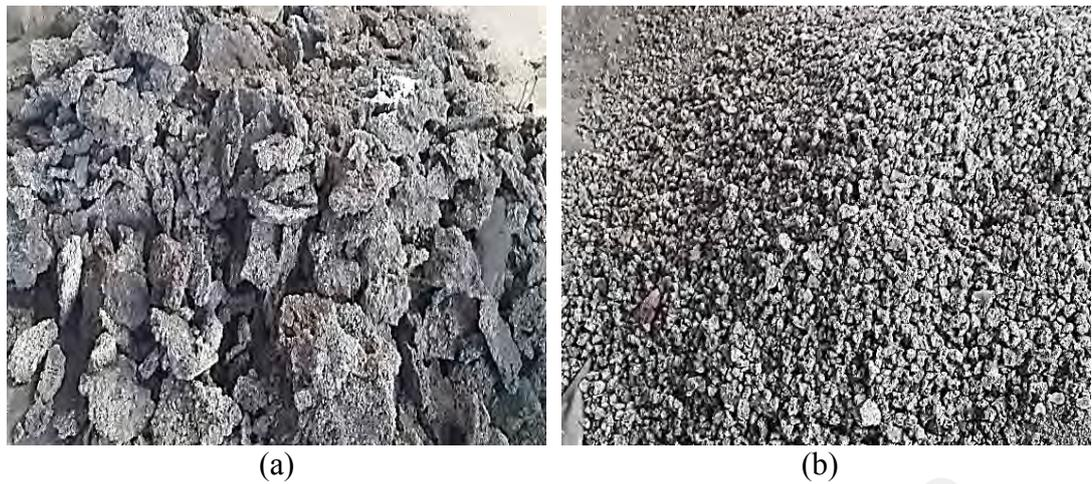
**Figure 2.7: OPBC aggregates: a) OPBC big lumps, b) Prepared OPBC for concrete**
