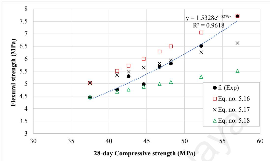
**Figure 5.11: Experimental and predicted flexural strength results of the concretes**
