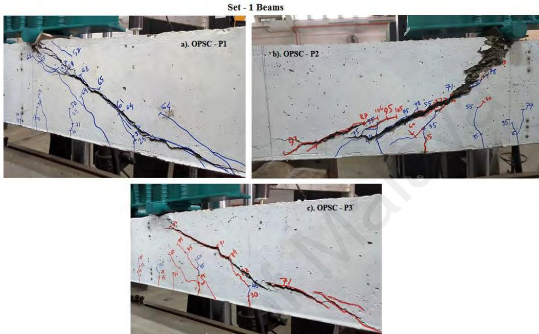
**Figure 9.8: Cracks pattern and Failure modes of the set-1 (OPS) lightweight weight concrete beams**
