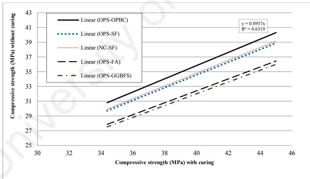
**Figure 3.5: The relationship between compressive strength of OPS-OPBC concrete with and without curing and comparison with OPS concrete containing silica fume (OPS-SF), normal concrete containing silica fume (NC-SF), OPS concrete containing fly ash (OPS-FA) and OPS concrete containing GGBFS (OPS-GGBFS)**
