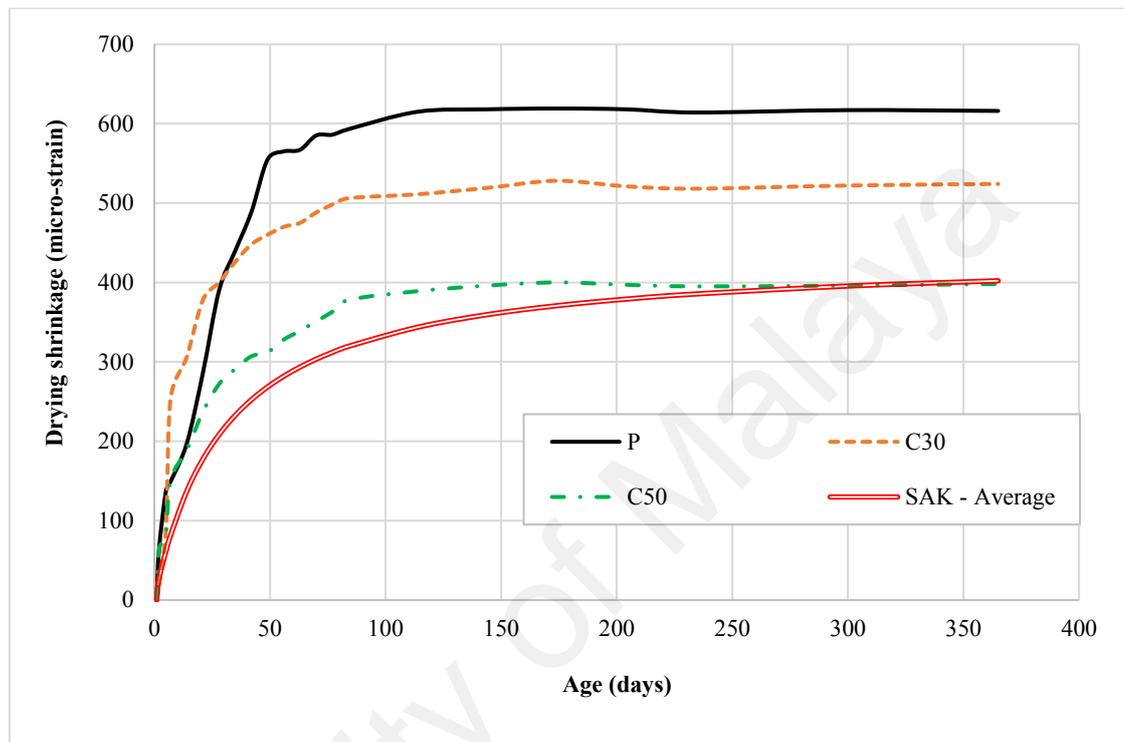
**Figure 8.9: Development of drying shrinkage (Experimental and average SAK model predictions)**
