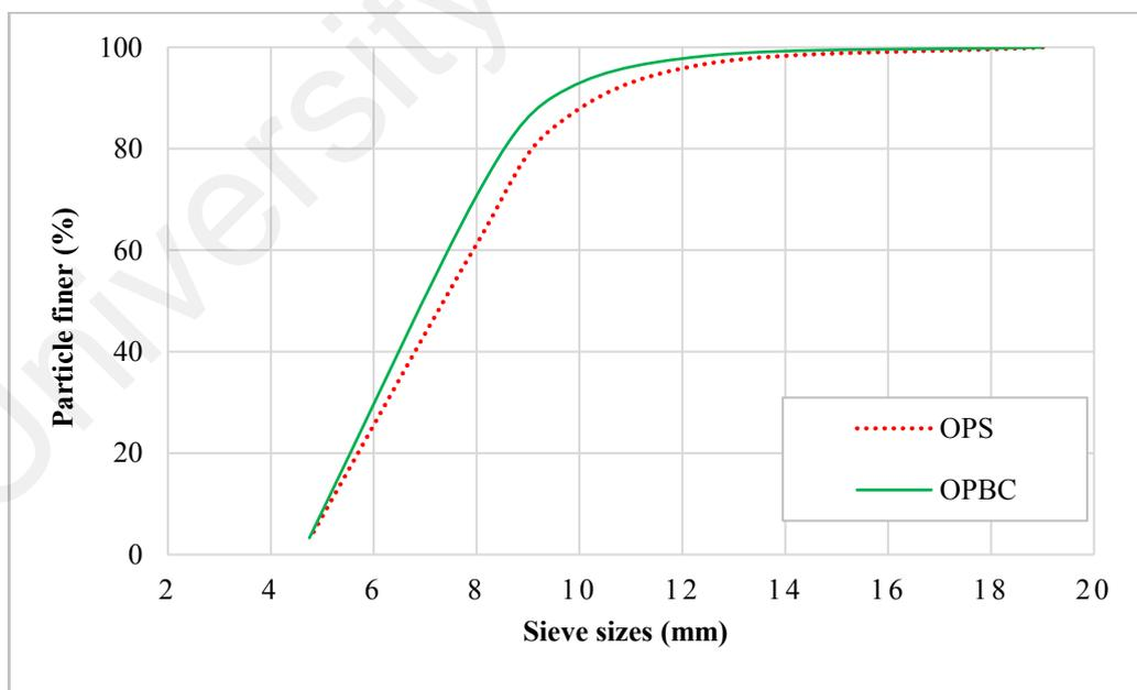
Figure 4.2: Grading of OPS and OPBC aggregates
