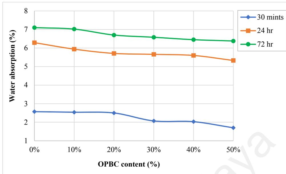
**Figure 3.8: Relationship between OPBC content and water absorption**
