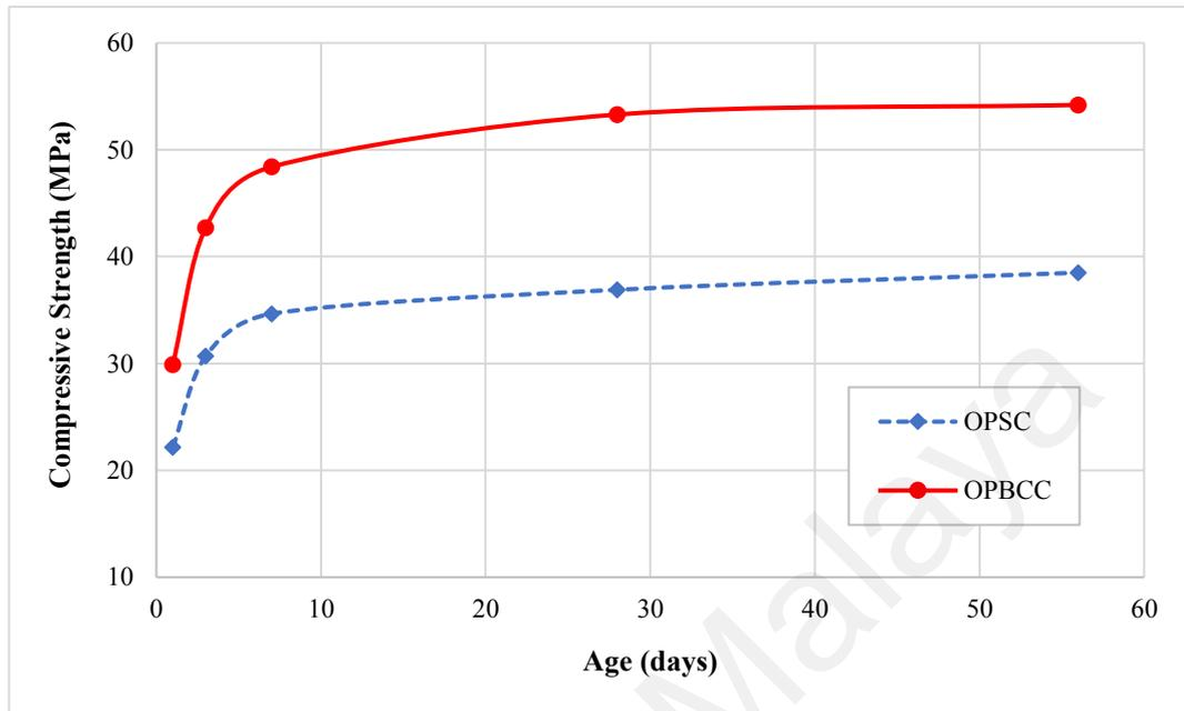
**Figure 4.3: Development of compressive strength**
