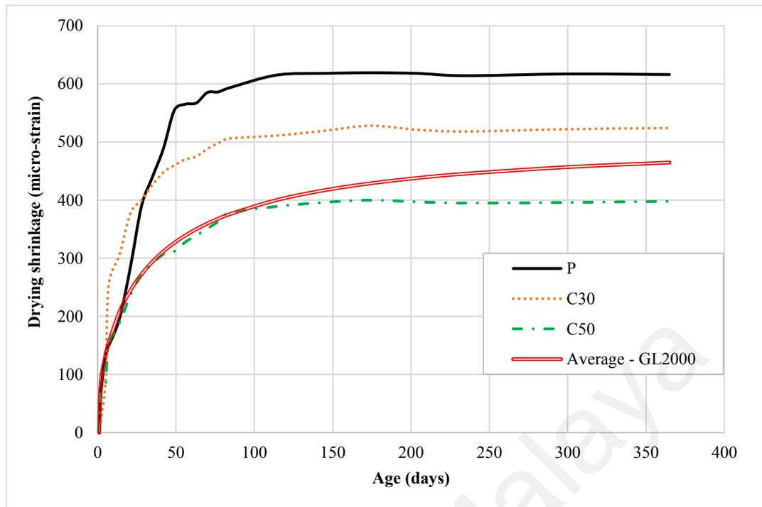
**Figure 8.6: Development of drying shrinkage (Experimental and average GL2000 predictions)**
