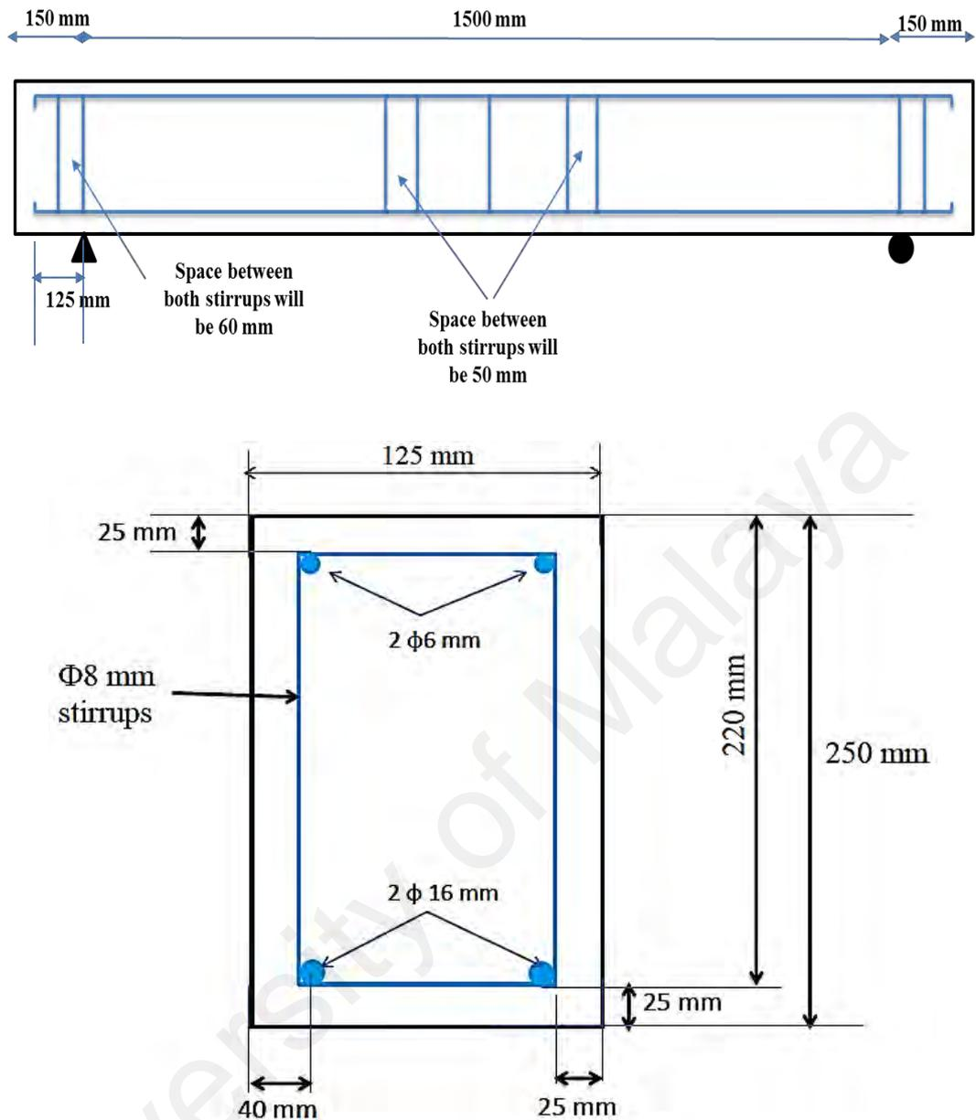
**Figure 9.1: Reinforcement details of the beams without shear reinforcement**
