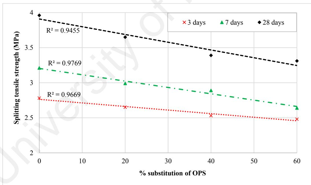
**Figure 5.8: Relationship between the splitting tensile strength and the substitution of OPS**
