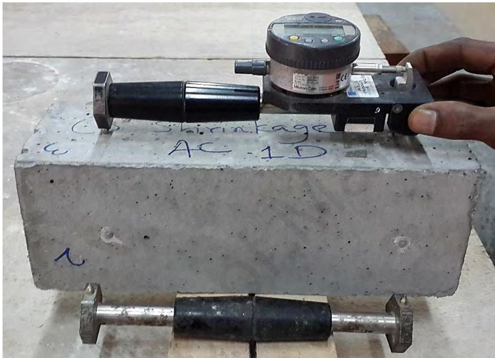
**Figure 6.3: The image of the measurement of drying shrinkage**
