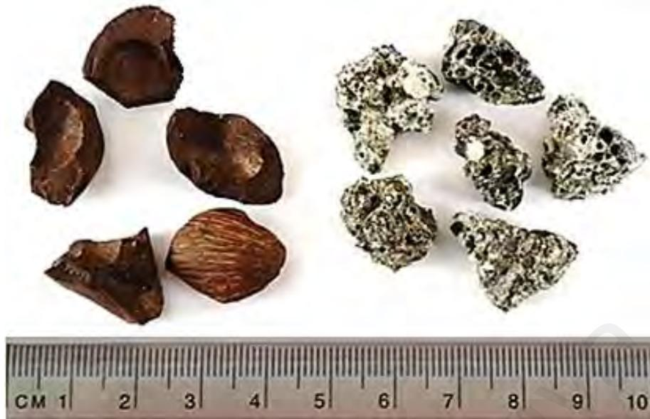
**Figure 3.1: Oil palm shell (left) and oil-palm-boiler clinker (right)**
