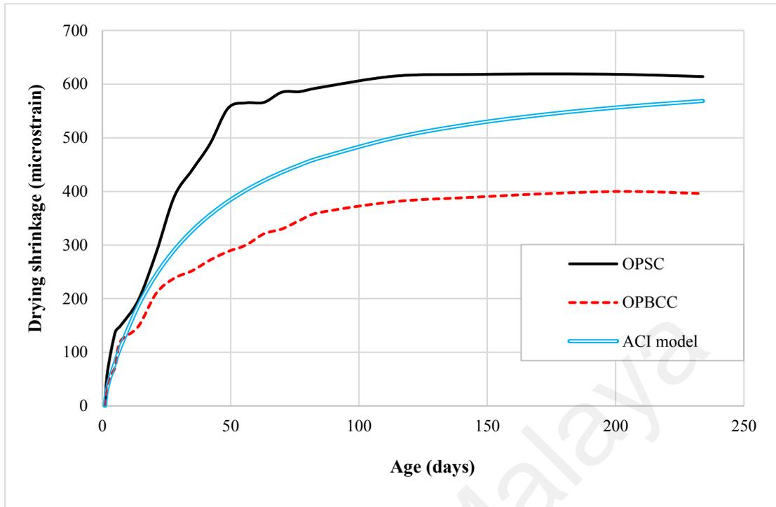
**Figure 4.5: Drying shrinkage strain development of concretes**
