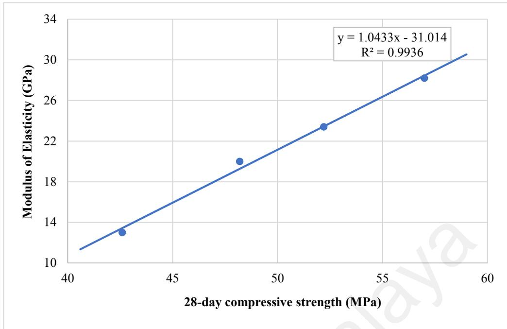
**Figure 5.12: Relationship between the modulus of elasticity and 28-day compressive strength**
