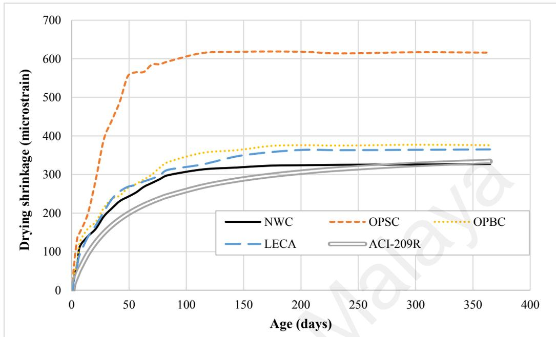
**Figure 7.7: Development of drying shrinkage with average predicted results under 7-day moist curing condition**
