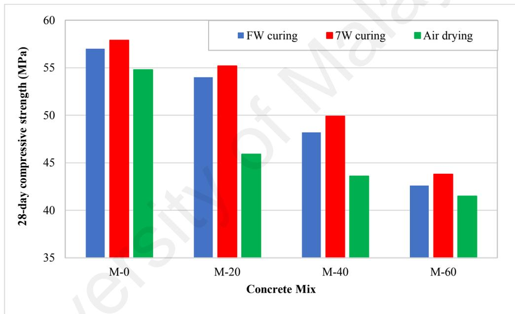
**Figure 5.5: 28-day compressive strength with and without curing**
