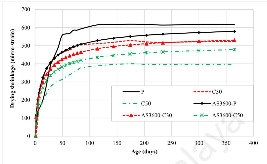
**Figure 8.7: Development of drying shrinkage (Experimental and AS3600 model predictions)**
