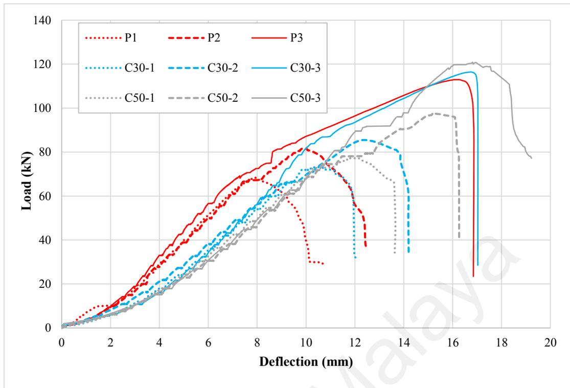
**Figure 9.6: Structural behaviour of all the beams without shear reinforcement**
