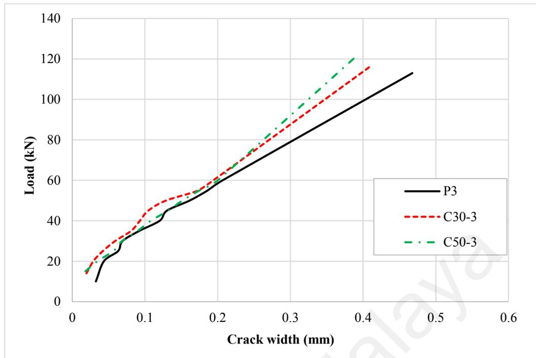
**Figure 9.13: Development of cracks widths of Grade 45 concrete beams**
