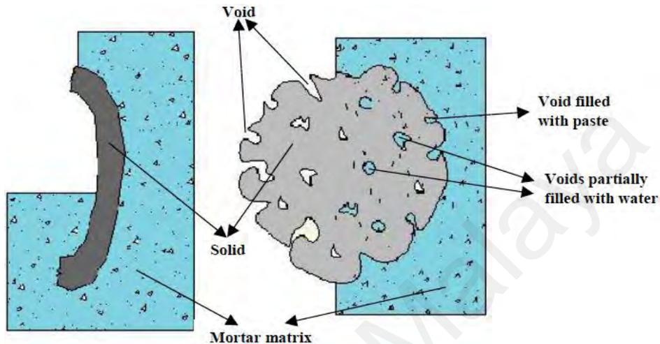
**Figure 3.4: Surface texture of OPS and OPBC aggregates with mortar matrix**
