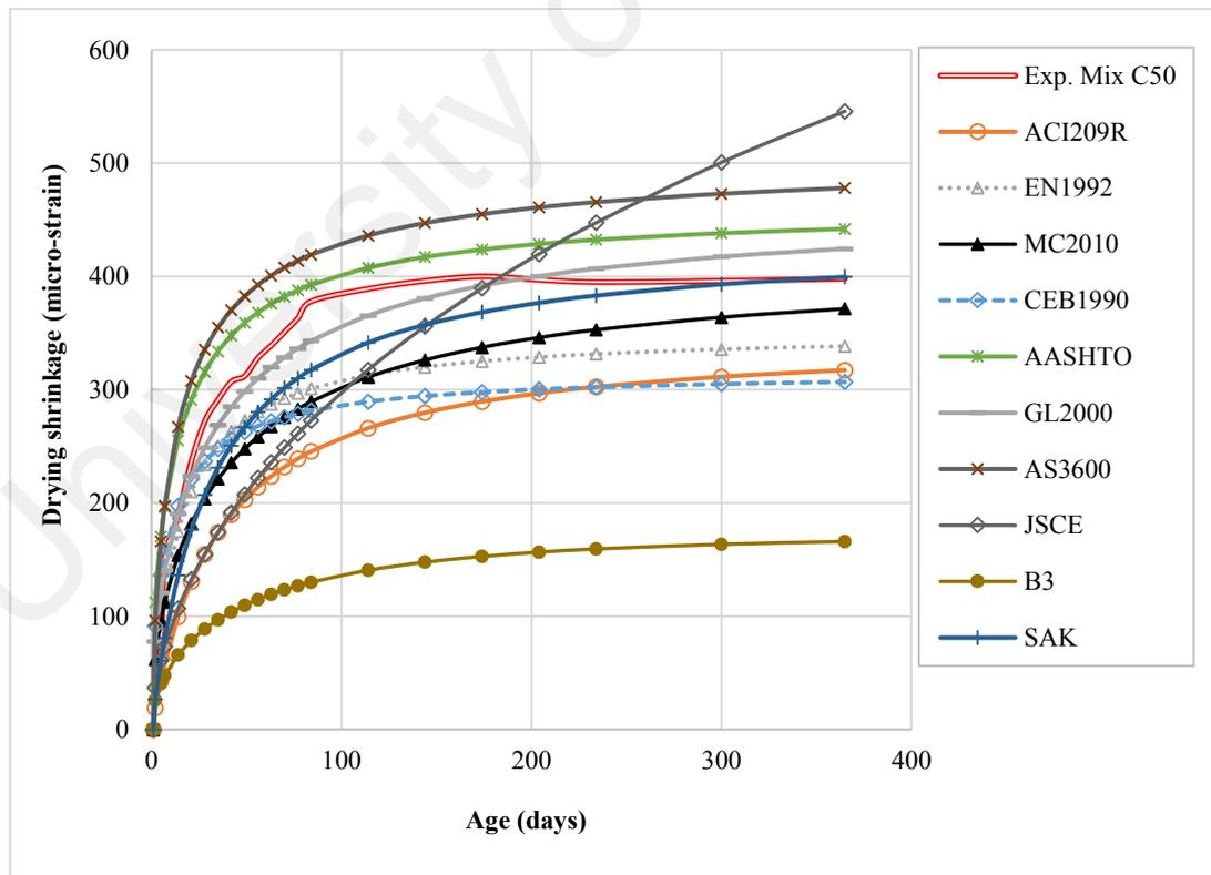
Figure 8.13: Comparison of drying shrinkage of OPS-OPBC concrete (mix C50) to the prediction models
