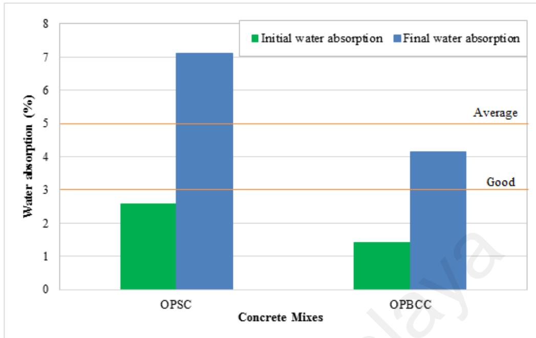
**Figure 4.4: Water absorption of concrete mixes**
