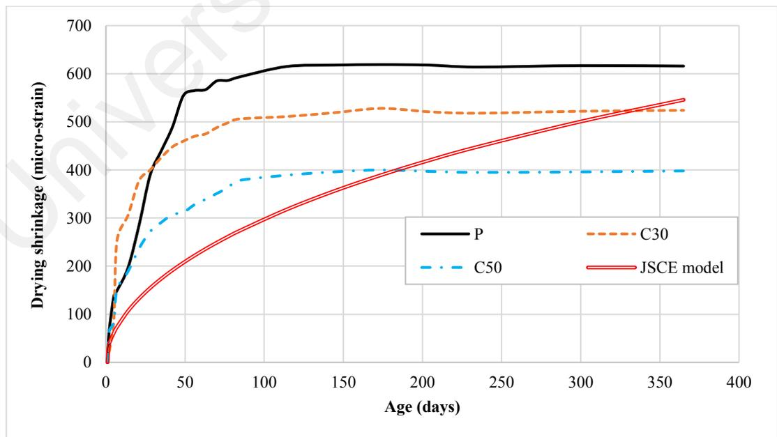
**Figure 8.8: Development of drying shrinkage (Experimental and average JSCE3600 model predictions)**
