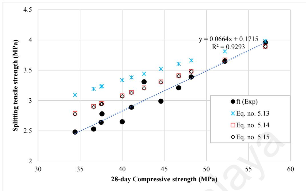
**Figure 5.9: Experimental and predicted splitting tensile strength of concretes**
