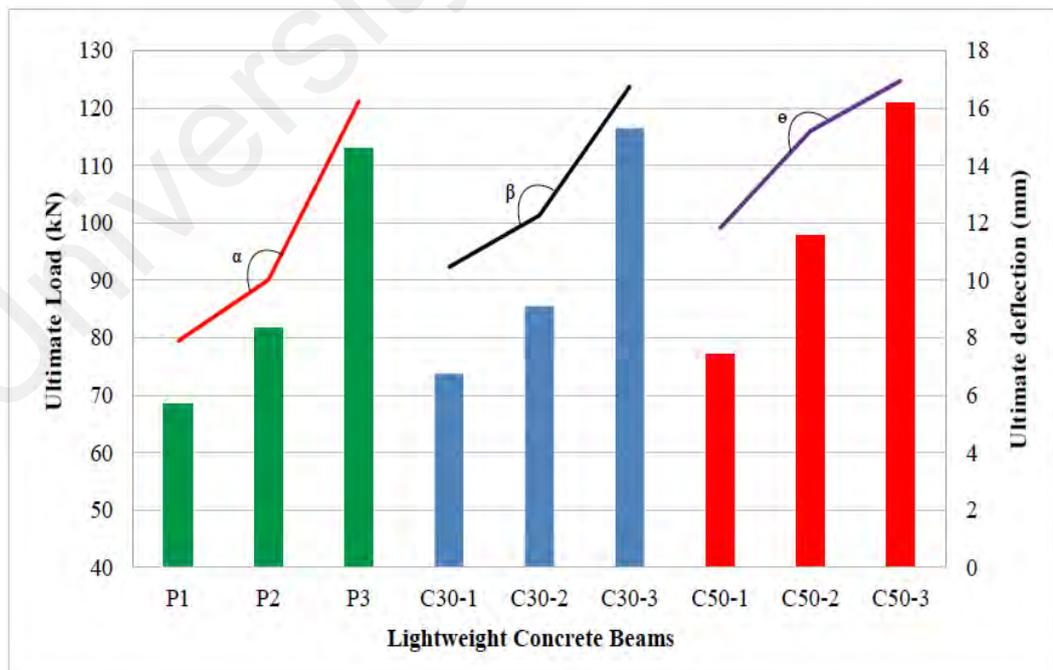
**Figure 9.7: Ultimate load capacity of all the beams with the respective deflections**
