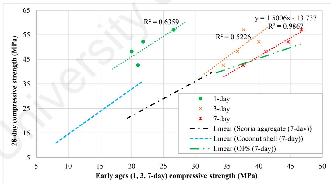
**Figure 5.4: The relationship between early ages and 28-day compressive strength of all mixes and comparisons with OPS lightweight concretes; scoria lightweight concrete; and coconut shell lightweight concretes**
