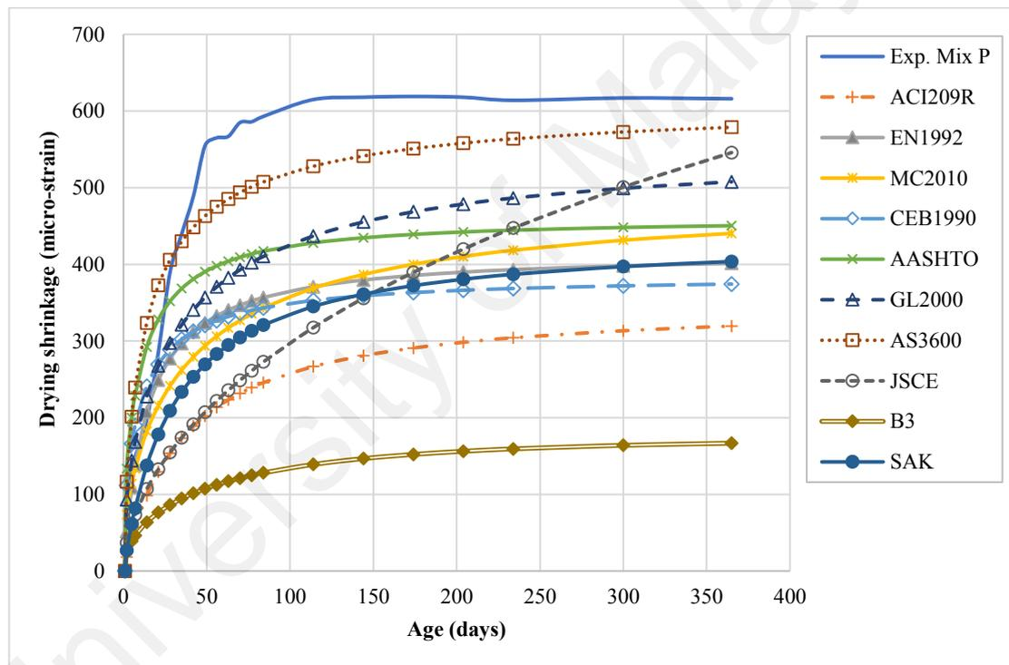
**Figure 8.11: Comparison of drying shrinkage of OPS concrete (mix P) to the prediction models**
