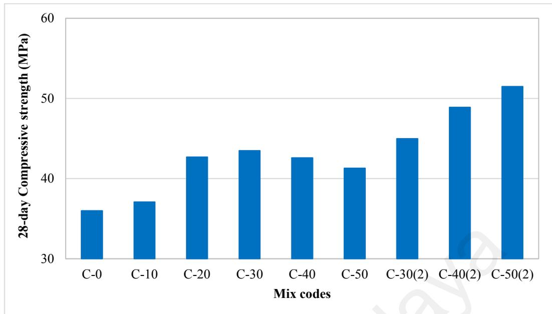
**Figure 6.4: 28-day compressive strength of concrete mixes**
