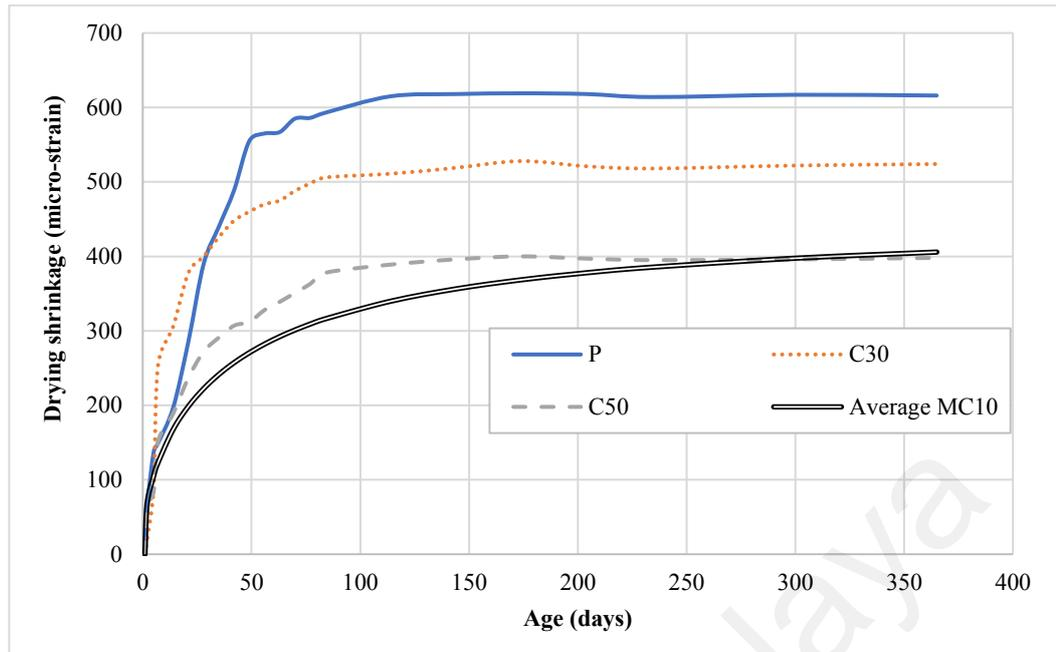
**Figure 8.3: Development of drying shrinkage (Experimental and average MC2010 (2011) prediction)**
