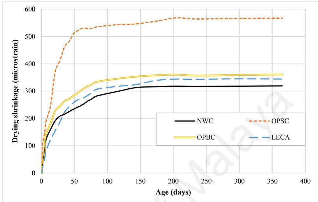
**Figure 7.2: Development of drying shrinkage strains under air-drying condition**
