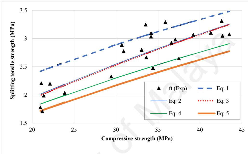
**Figure 3.6: Experimental and theoretical splitting tensile strength of all concrete mixes**
