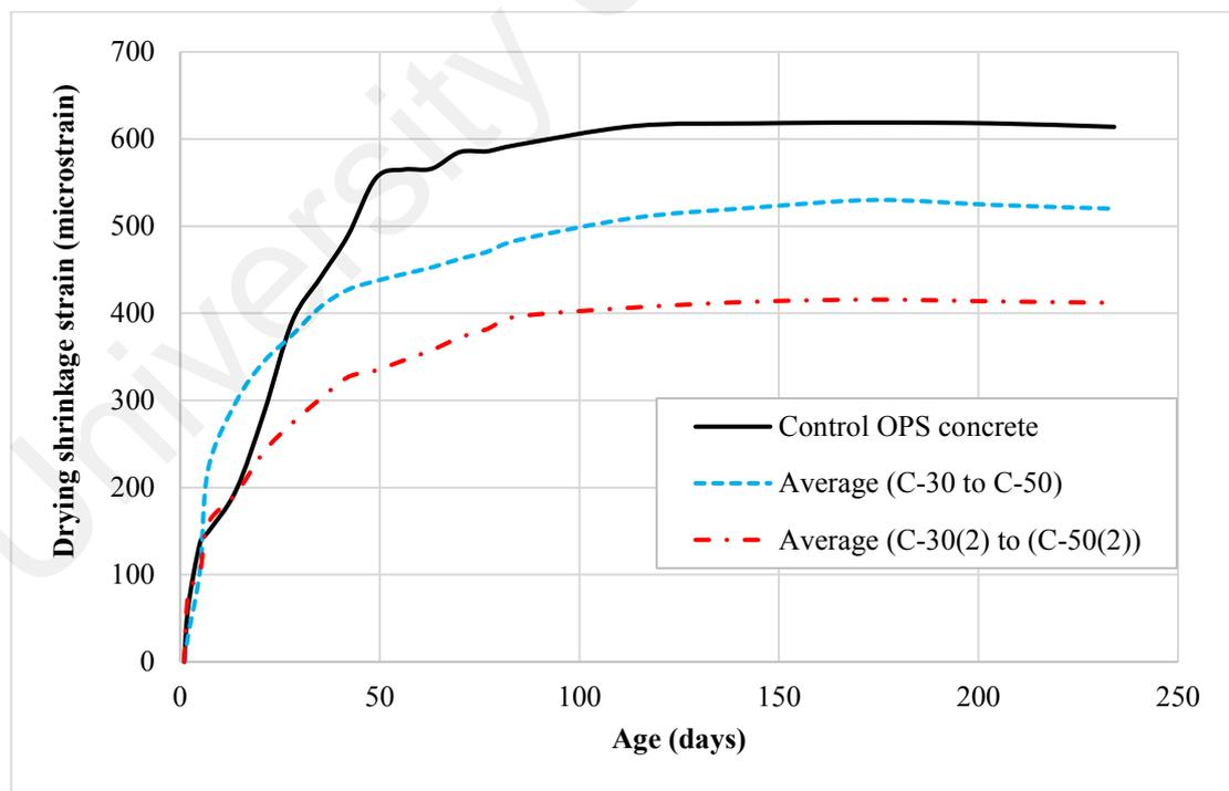
**Figure 6.13: Development of drying shrinkage of both set mixes under 7-day curing**
