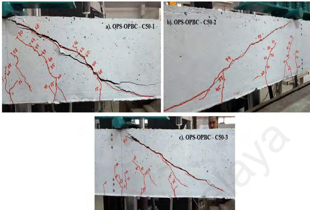
**Figure 9.10: Cracks pattern and Failure modes of the set-3 (OPS-OPBC50%) LWC beams**
