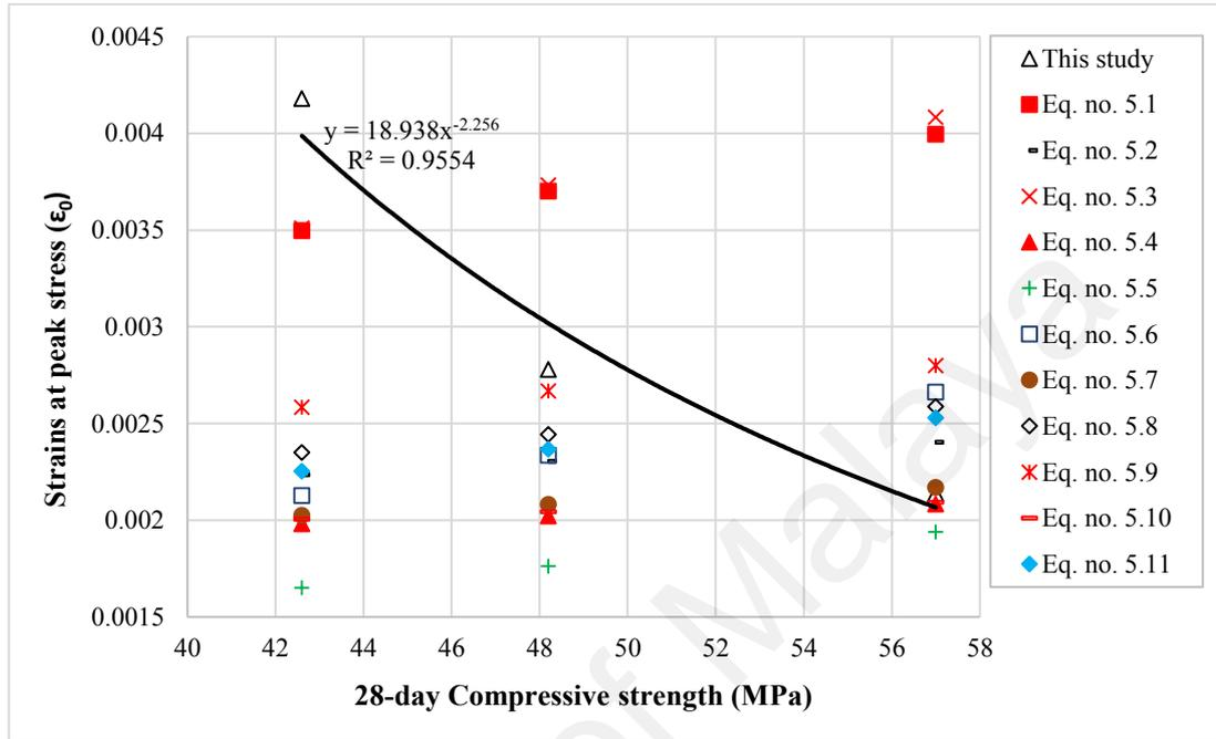
**Figure 5.7: Relationship between the 28-day compressive strength and strains at peak stress and comparison with predicted values**
