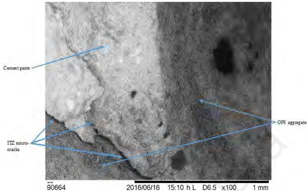
**Figure 7.4: A micro-cracks occurred during the drying of OPS concrete**
