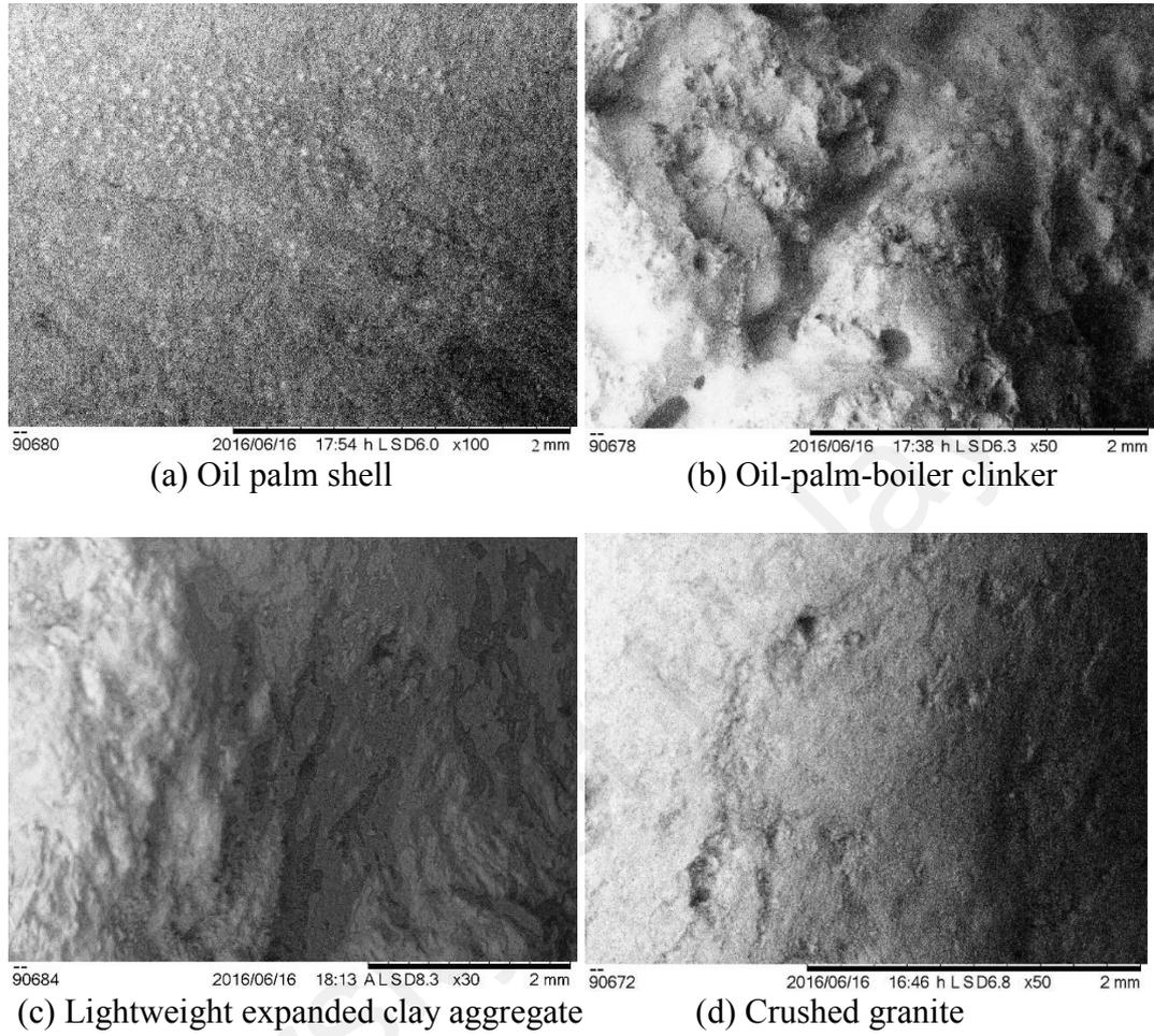
**Figure 7.3: Scanning Electronic Microscopic image of the aggregates**
