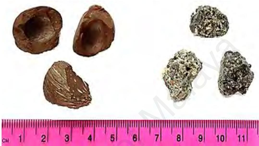
Figure 4.1: Oil palm shell (left) and oil-palm-boiler clinker (right)
