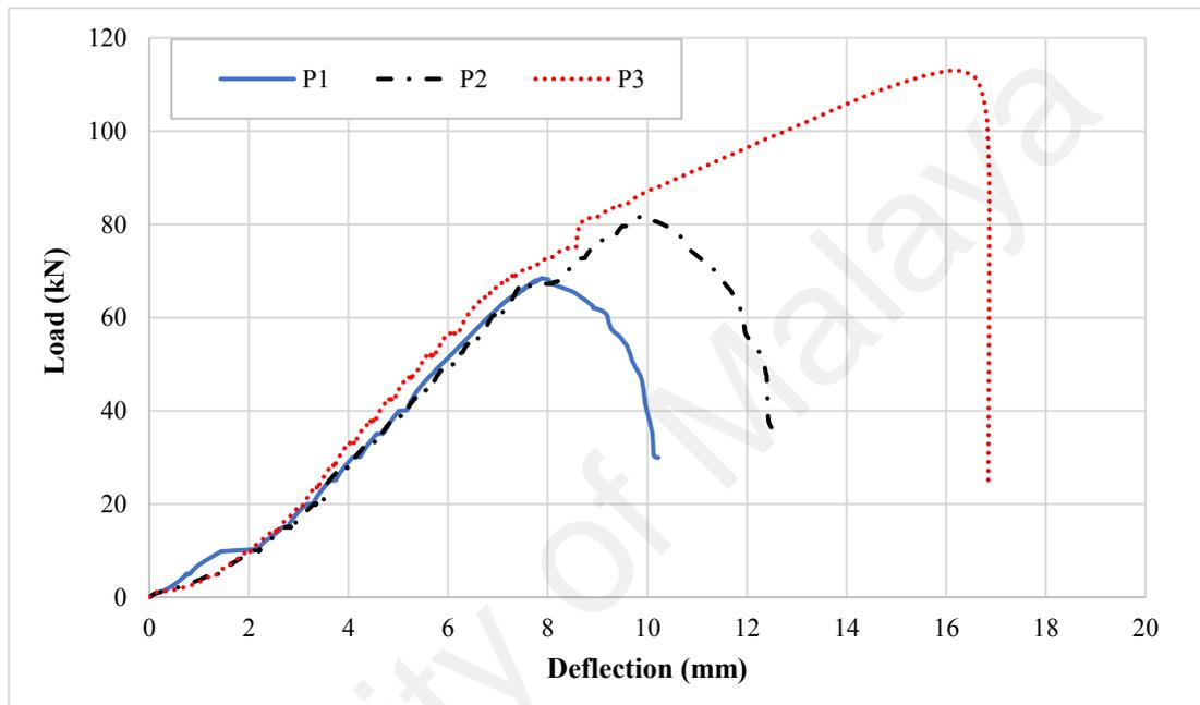
**Figure 9.3: Structural behaviour of OPS concrete beams (set-1) without shear reinforcement**
