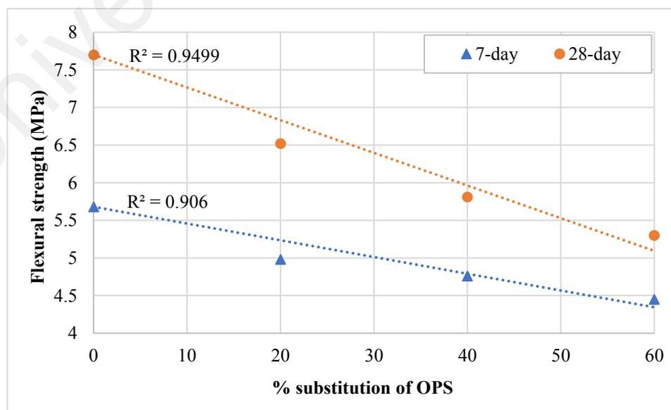
**Figure 5.10: Relationship between the flexural strength and the substitution of OPS**
