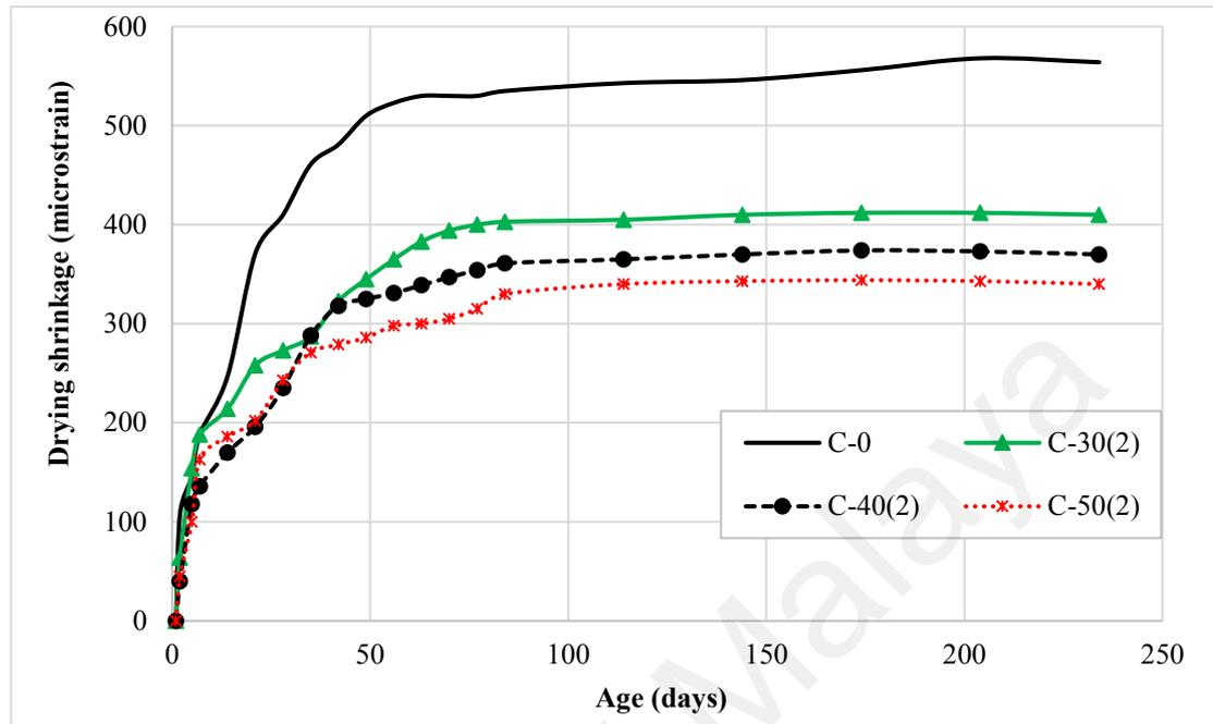
**Figure 6.7: Development of drying shrinkage of set (2) concrete mixes**
