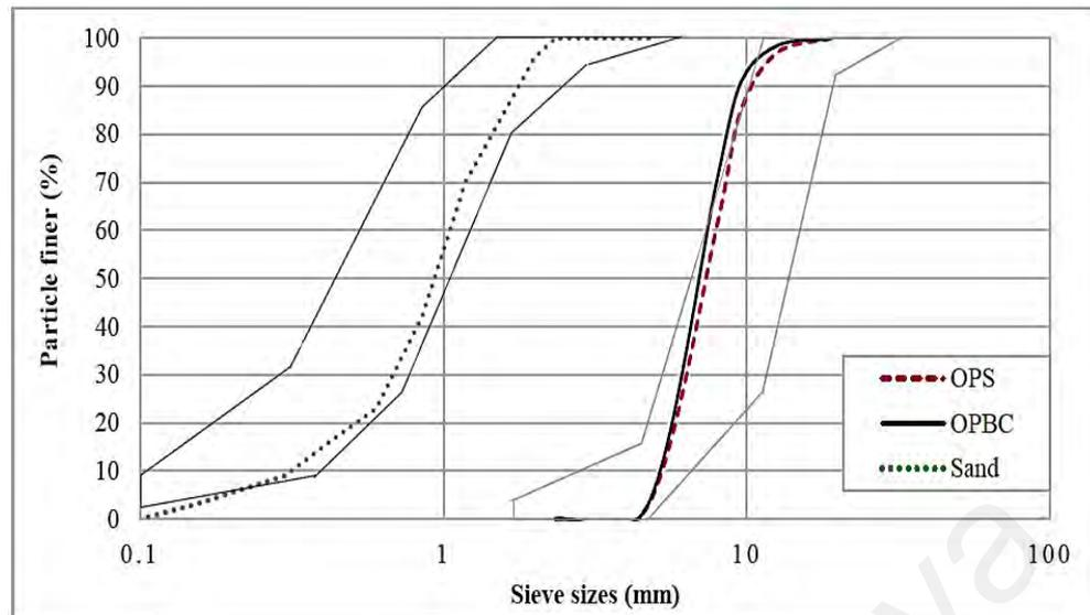
Figure 6.1: The grading of the aggregates as per limits specified by ASTM C-33
