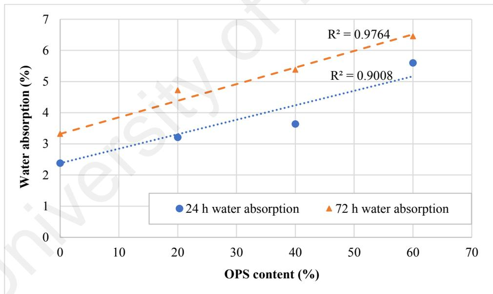
**Figure 5.14: Relationship between water absorption and the OPS content**
