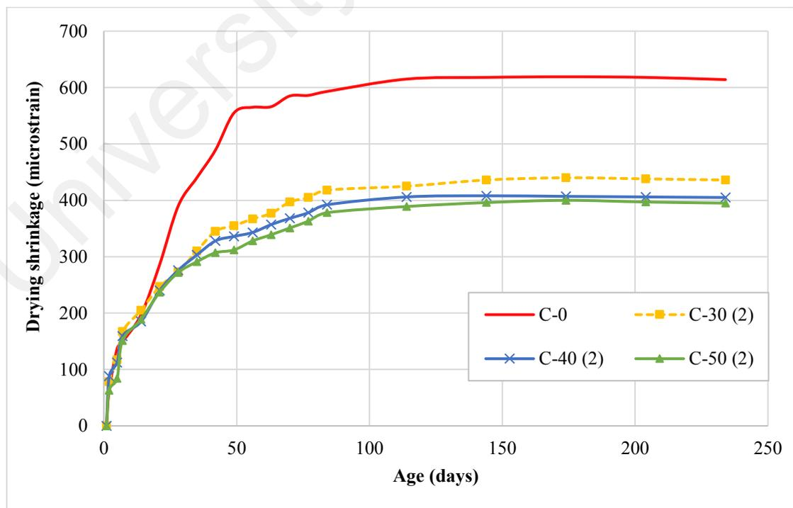
**Figure 6.12: Drying shrinkage of OPS-OPBC mixtures at reduced water/cement ratios**
