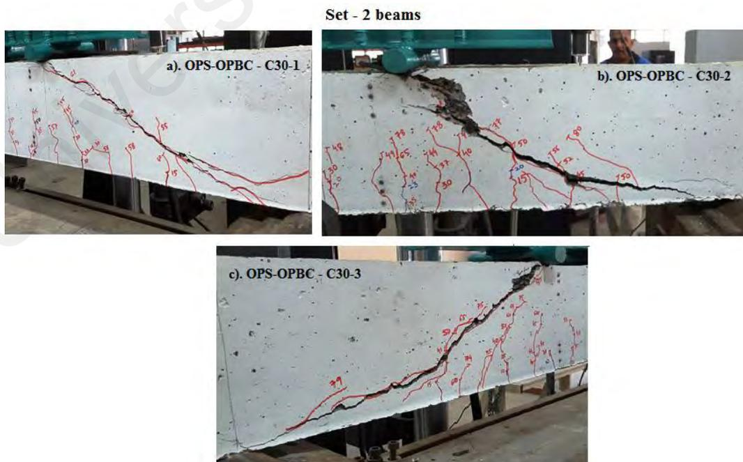
**Figure 9.9: Cracks pattern and Failure modes of the set-2 (OPS-OPBC30%) LWC beams**
