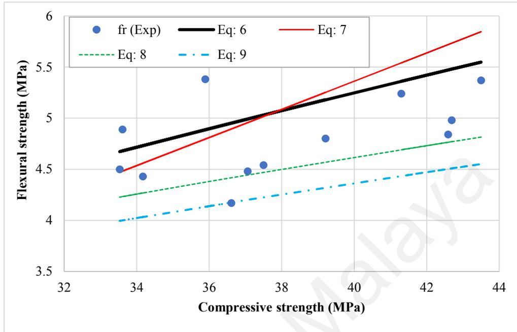
**Figure 3.7: Experimental and theoretical flexural strength results of all concrete mixes**
