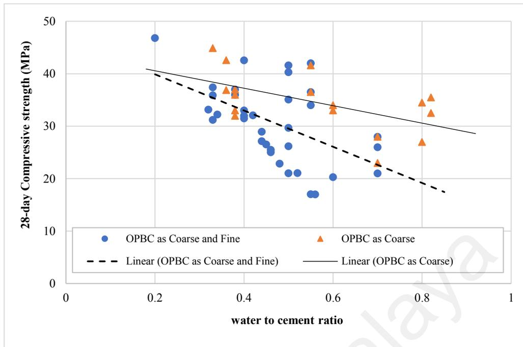
**Figure 2.8: Compressive strengths of OPBC concrete at different w/c ratios**
