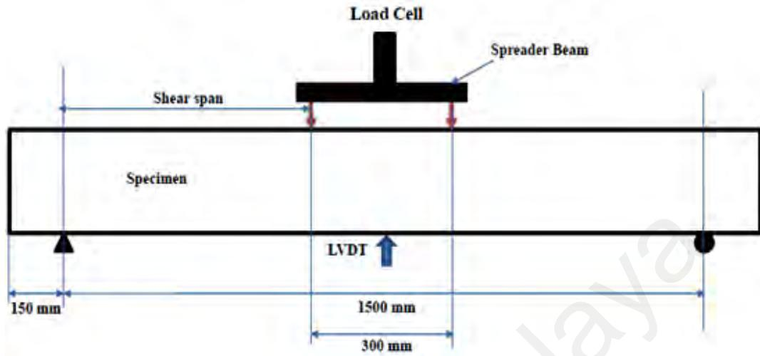
**Figure 9.2: Test setup and Instrumentation**
