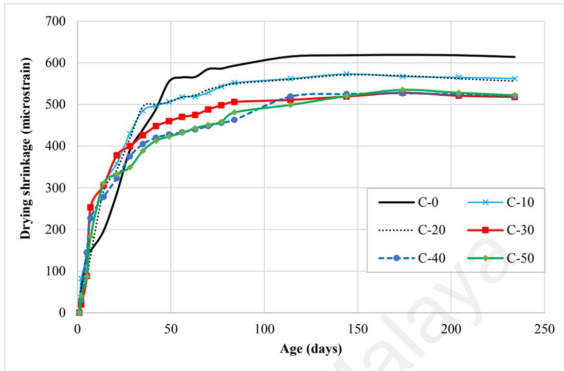
**Figure 6.11: Drying shrinkage of OPS-OPBC mixtures after 7 days curing**
