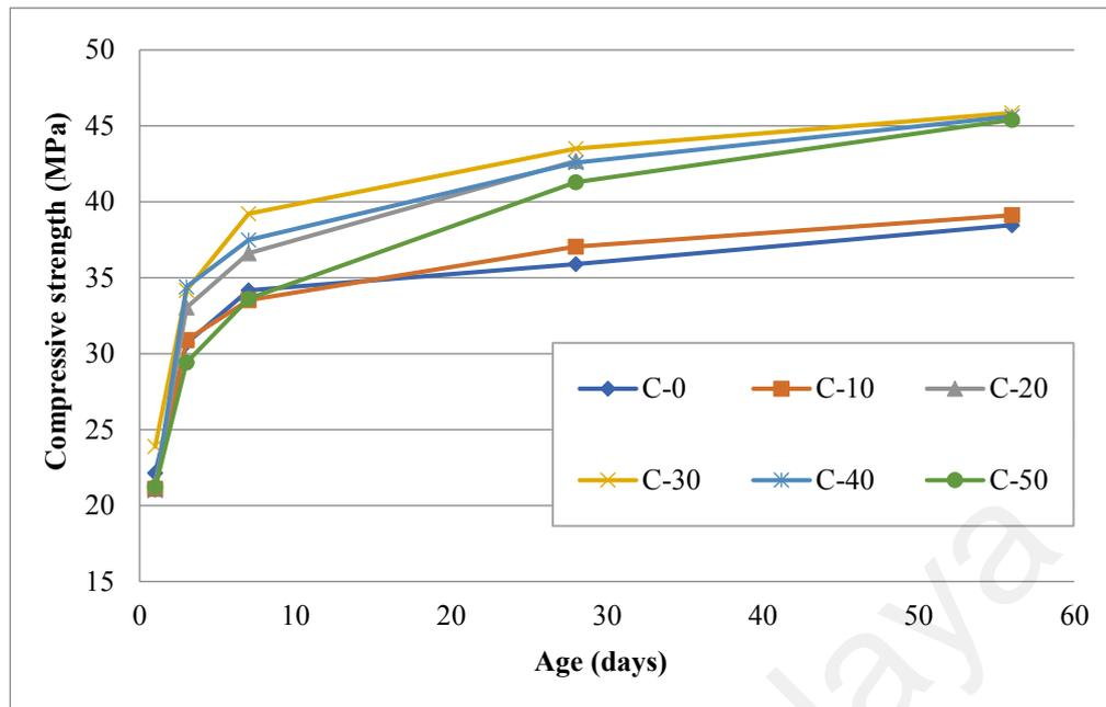
**Figure 3.3: Compressive strength development of concrete**
