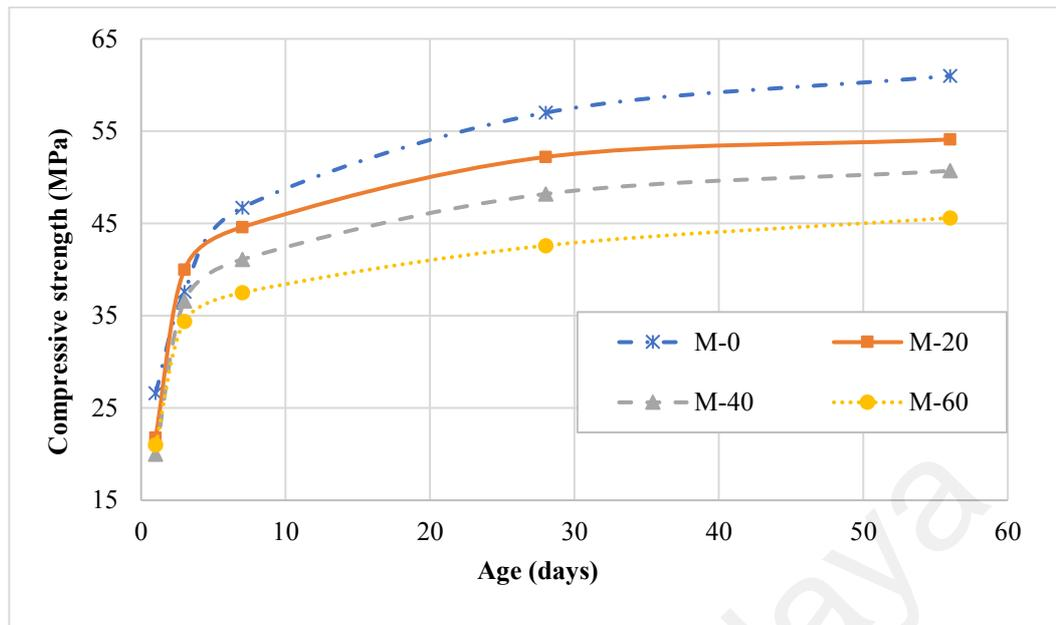
**Figure 5.3: Development of compressive strength of the concrete mixes**
