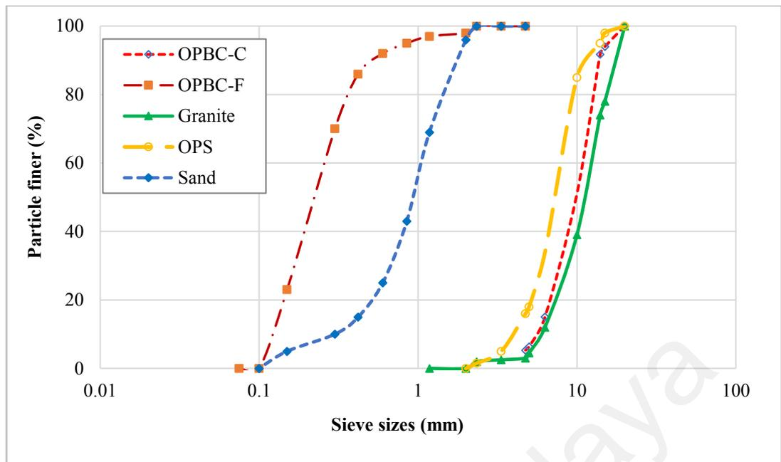
**Figure 2.6: Particle size distribution of the OPBC compared with other LWA reported in the literature**
