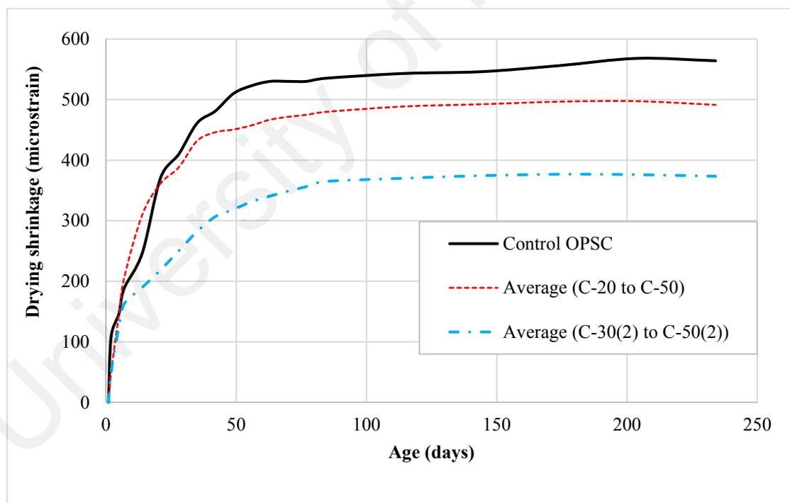
**Figure 6.8: Development of dying shrinkage of both sets mixes**
