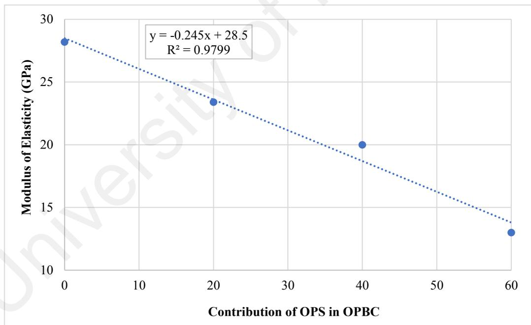
**Figure 5.13: Relationship between the modulus of elasticity and contribution of OPS in OPBC**
