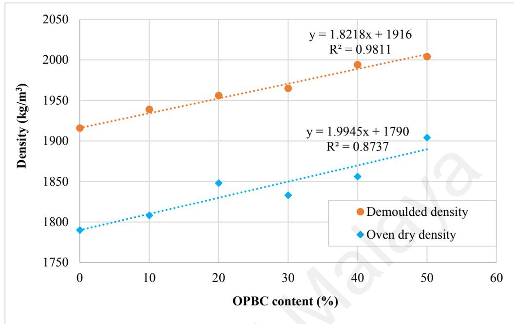
**Figure 3.2: Relationship between density and OPBC content**
