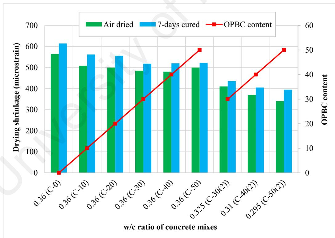
**Figure 6.10: Drying shrinkage and OPBC content versus the w/c ratio**
