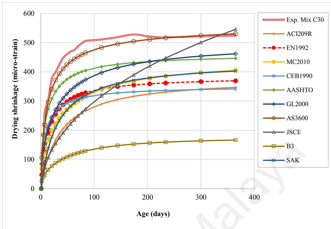
Figure 8.12: Comparison of drying shrinkage of OPS-OPBC concrete (mix C30) to the prediction models
