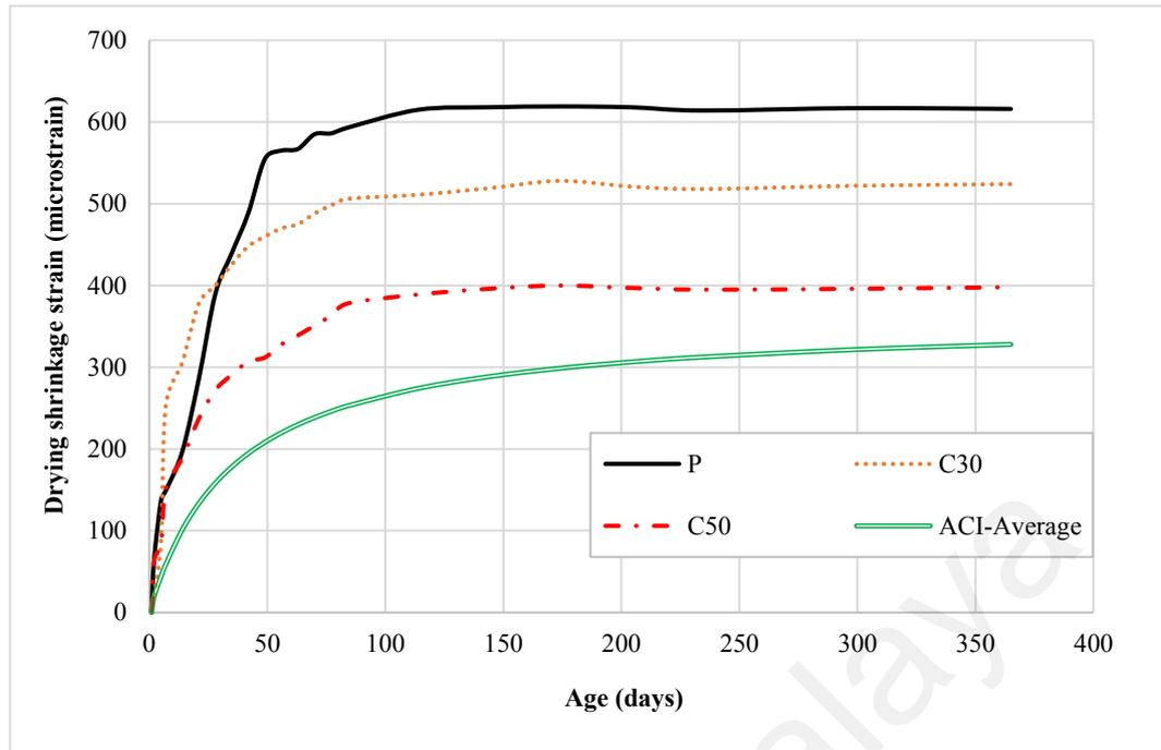
**Figure 8.1: Development of the drying shrinkage (Experimental vs. average ACI209R (2008) prediction)**
