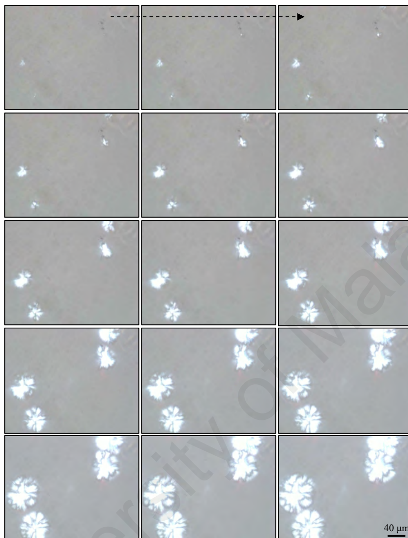
Figure 4.21 Micrographs captured after 5 min growing of P(3HB-co-8mol% 3HHx) spherulites at T_c = 110^\circ\text{C} at 60 s time interval every micrograph. Magnification 50×
