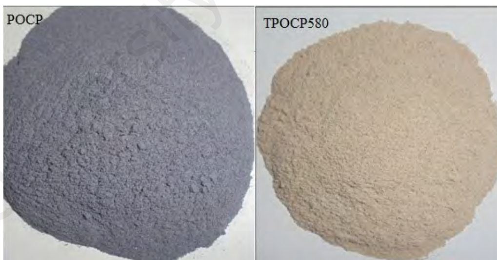
Figure 4.9: Color change due to thermal activation
