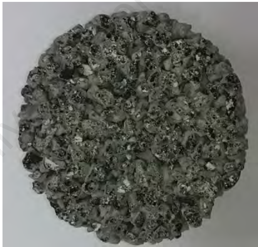
Figure 2.6: Cross section of pervious concrete (Ibrahim & Razak, 2016)
