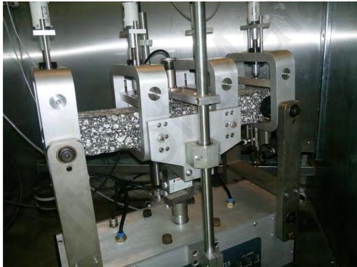
**Figure 3.7: Test arrangement in four point bending apparatus**
