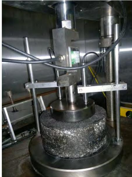
**Figure 3.9: Dynamic creep test arrangement**
