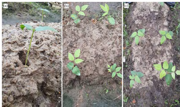
Figure 4.20: Images of the field trial, (a) PVA/KF on the soil at 3 DAS, (b) cross-linked PVA/KF after 7 DAS, (c) PVA/KF after 7 DAS.
