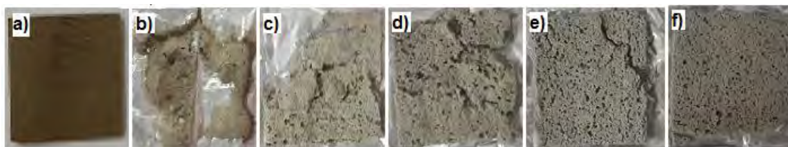
Figure 4.15: The appearance of control and cross-linked PVA/KF composites before (a) and after 24 hours of water absorption (b-f), in which (a) PVA/KF, (b) PVA/KF, (c) PVA/KF/MDI-2.5%, (d) PVA/KF/MDI-5.0%, (e) PVA/KF/MDI-7.5%, (f) PVA/KF/MDI-10.0%.
