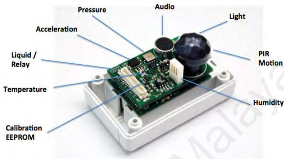
Figure 1.2 : Sensor board for firefly environment
