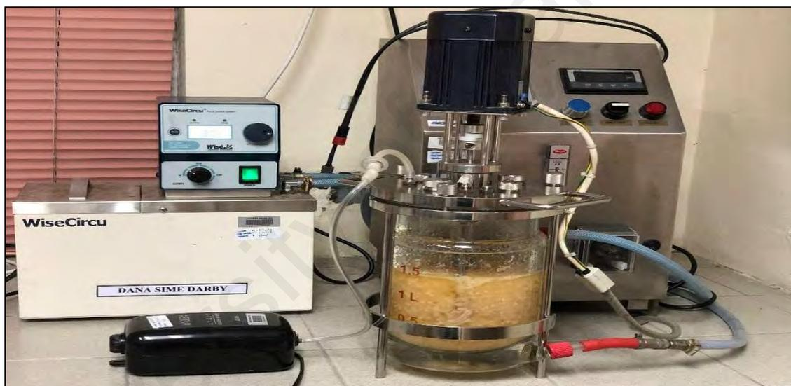
**Figure 4.10:** Experimentation set up for up-scaling the bioremediation of diesel.
