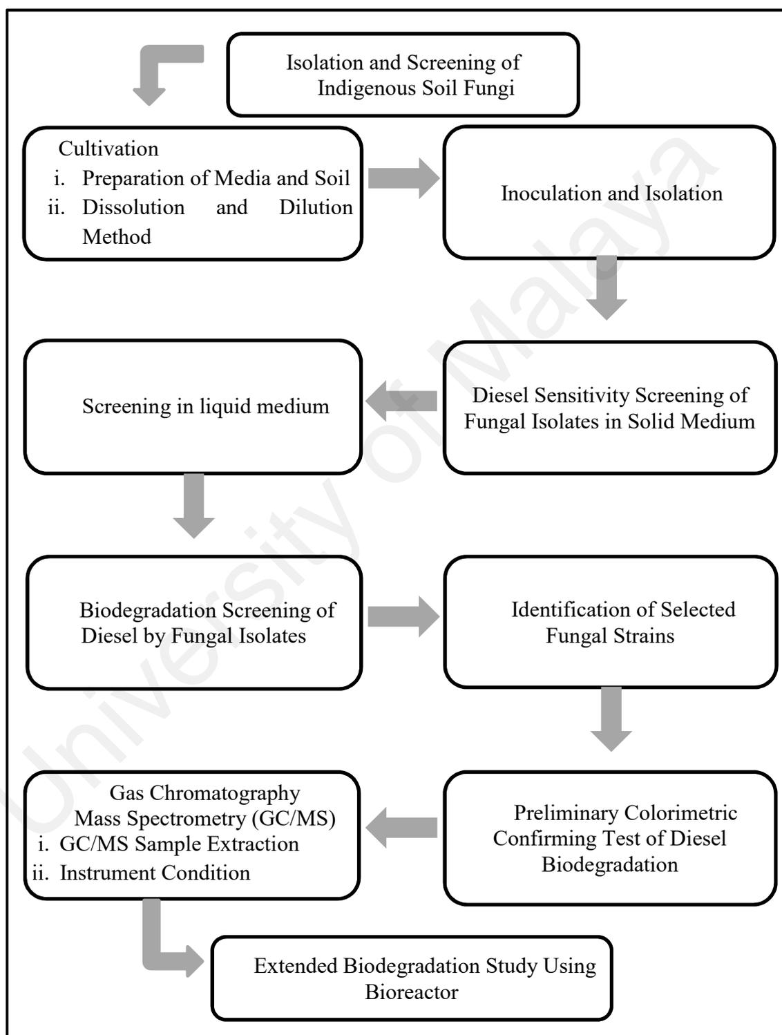
**Figure 3.1:** Schematic diagram for laboratory work.
