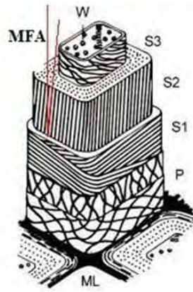
Figure 2.1(a): Schematic fiber structure: consisting different layers of cell wall (middle lamella, primary and secondary cell walls (P, S1, S2, S3) and cell lumen (W))
