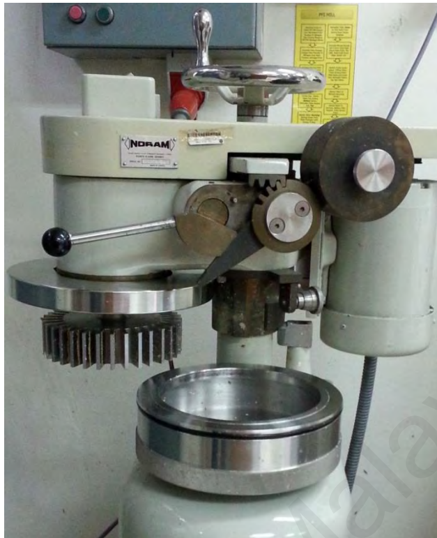
Figure 2.5: PFI laboratory beating mill
