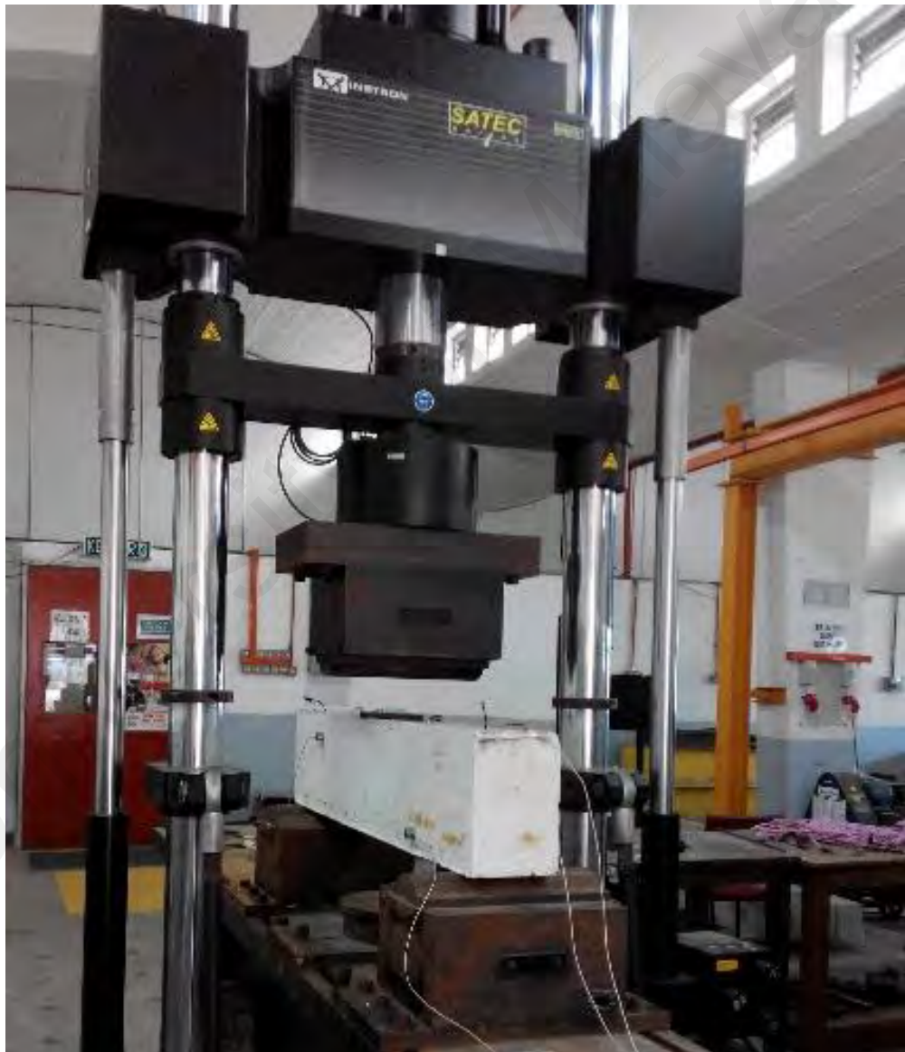
Figure 3. 10: Universal testing machine (INSTRON Satec Series of 600 kN)
