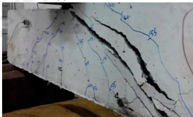
(c) damage localization
