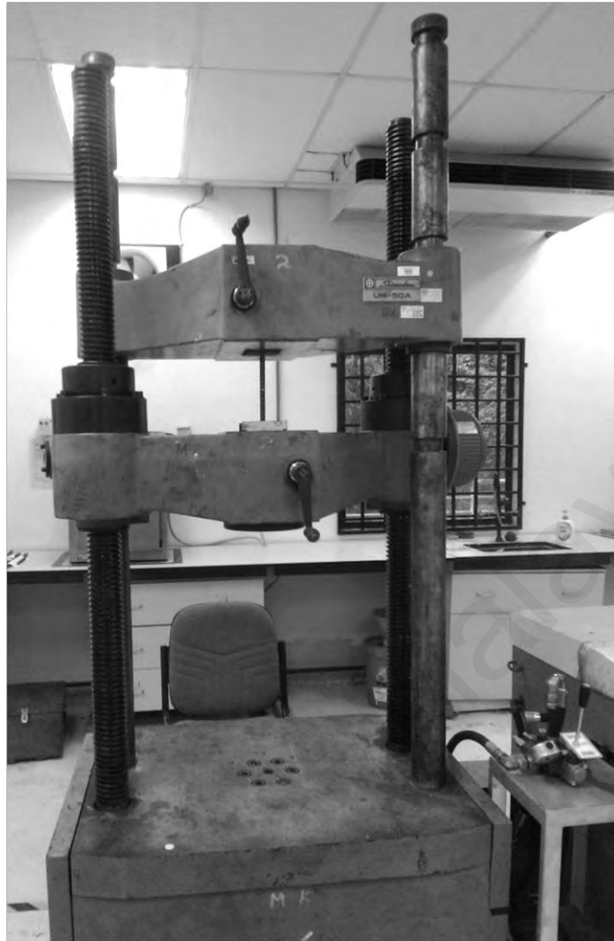
Figure 3. 15: Tensile test of the reinforcement
