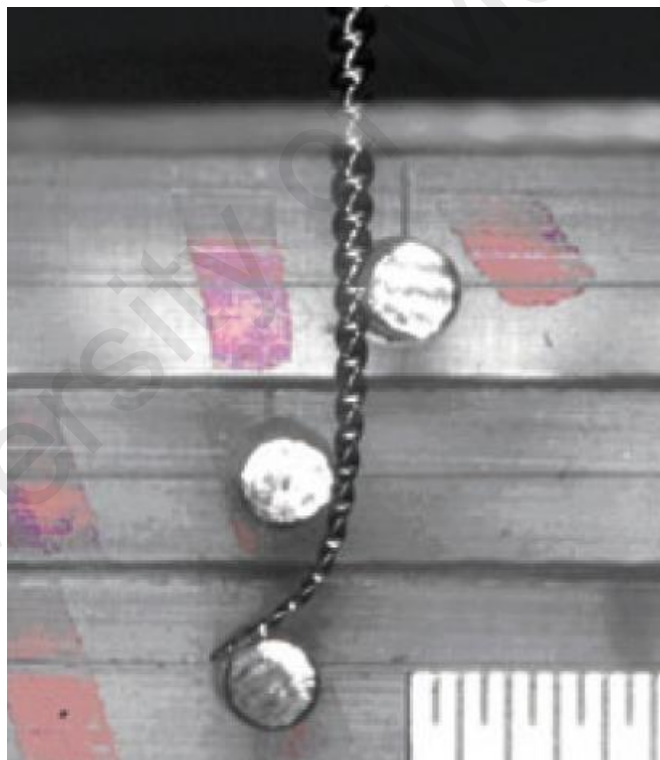
Figure 3.7 An example of 3-point Bending with Stainless Steel Pins (Cheung & Darvell, 2007a).
