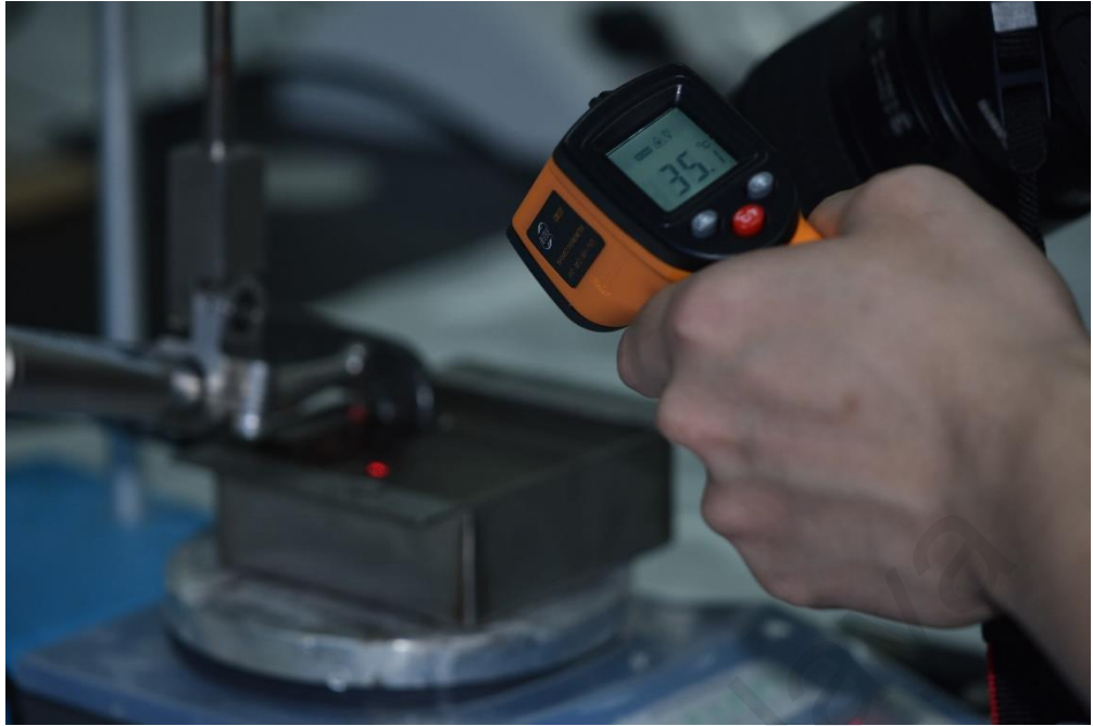
Figure 4.4 Temperature of stainless steel canal monitored by digital laser infrared temperature sensor.
