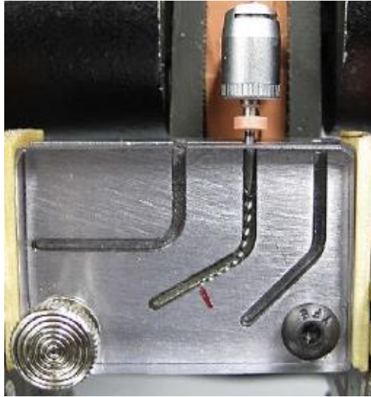
Figure 3.10 Metal block with 1.5 mm wide artificial canal (Larsen et al. , 2009).
