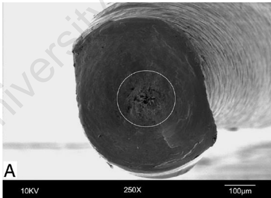
Figure 3.3 SEM of fractured surface of instrument circular abrasion marks that caused by torsional fracture (Alcalde et al. , 2017).
