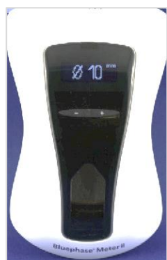
Figure 4.18: Dental radiometer used to measure LCU irradiance
