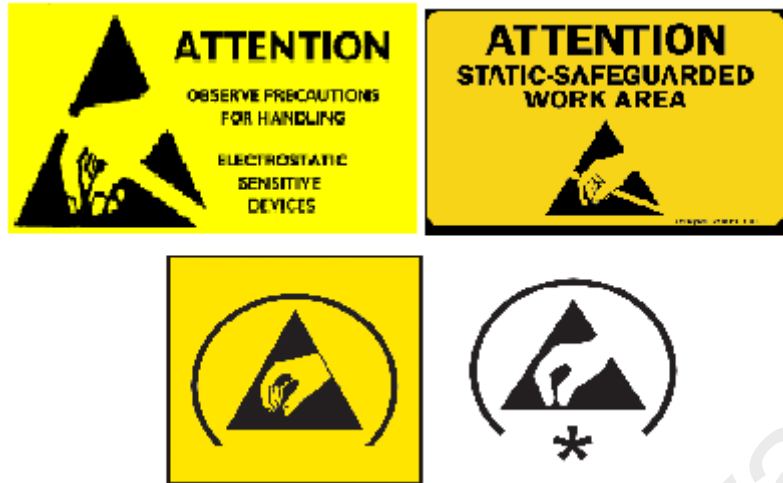
Figure 2.3: Examples of ESD hazard labels
