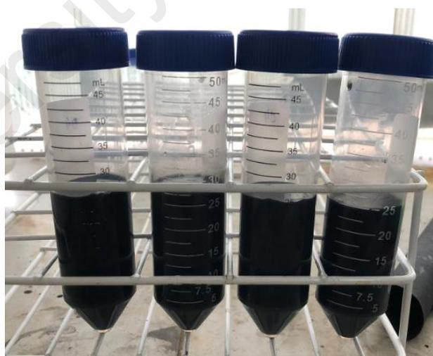
**Figure 3.3 GO mixture shake by hand to washing after centrifuged for 5 minutes.**
