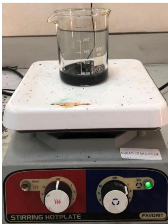
**Figure 3.8 GO-NiO powder dissolved in the distilled water and PEO was added into solution.**
