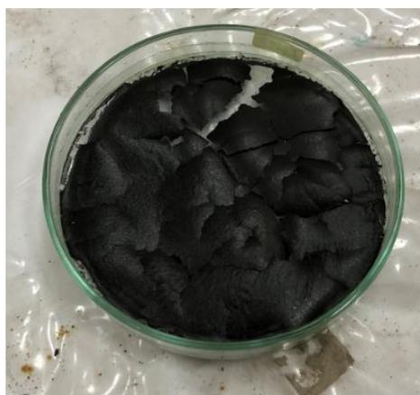
**Figure 3.5 Flakes of GO-NiO after drying in the oven for 18 hours.**
