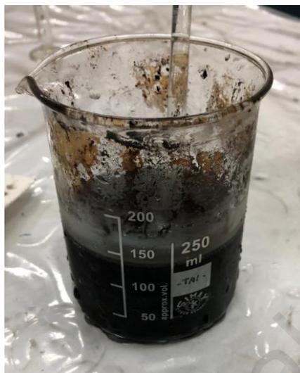
**Figure 3.1** The mixture solution of graphite and potassium permanganate.
