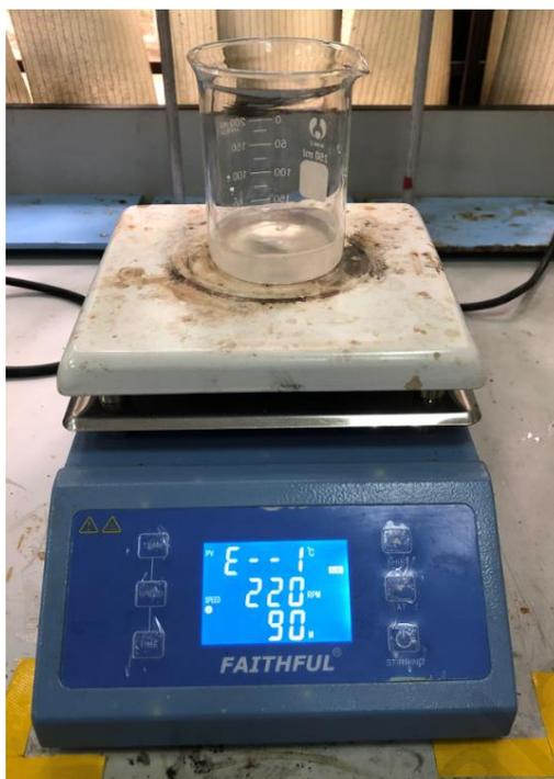
**Figure 3.7 PEO dissolved in distilled water and stirred for 4 hours to obtained homogenous solution.**
