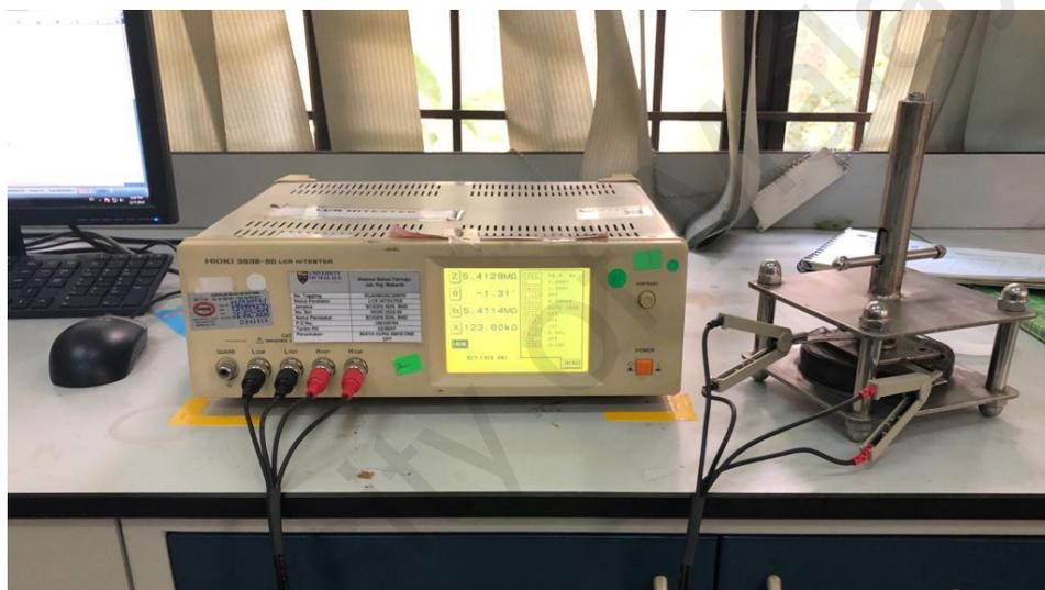
**Figure 3.13 LCH Hitester for testing electrical properties of sample.**
