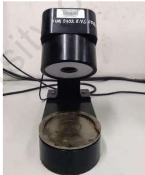
Figure 11: Four Ball Tribotester Arrangement
