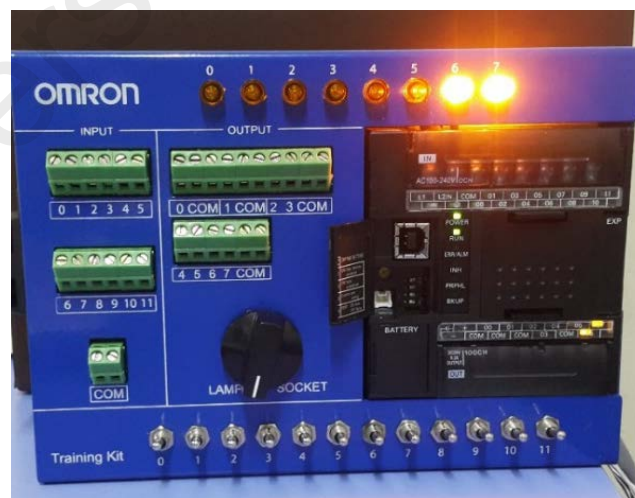
Figure 4. 19 Indicators are on as DC motors are in action
