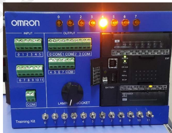
Figure 4. 17 The third motor receives the signal and running forward
