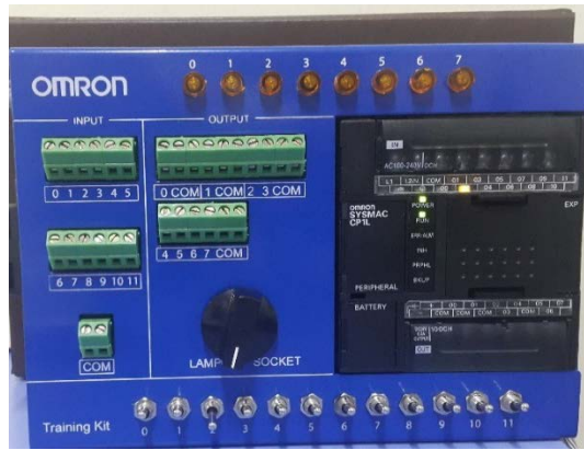
Figure 4. 20 Switch 2 activated to stop the system from running
