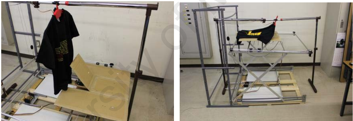
Figure 2. 4 Folding of clothes from hanging (source; (Miyamotoa et al., 2014))
