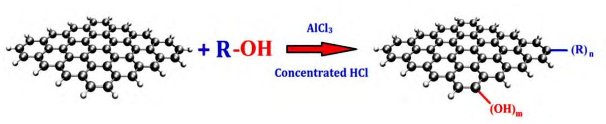
**Figure 4.23:** The experimental procedure for chemical-assisted functionalization of GNP with EG.
