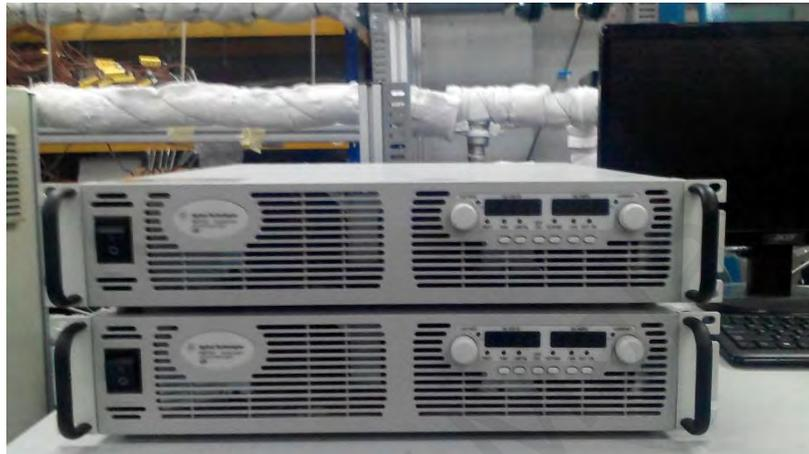
**Figure 3.13:** Photograph of the N8731A DC-power supplies.
