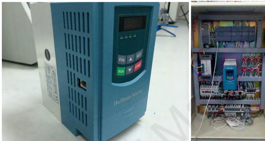
**Figure 3.9:** Photograph of the Hoffman Muller inverter.
