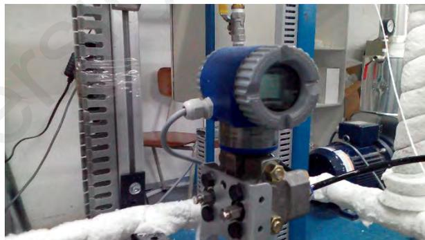
**Figure 3.11:** Photograph of the Differential Pressure Transducers.
