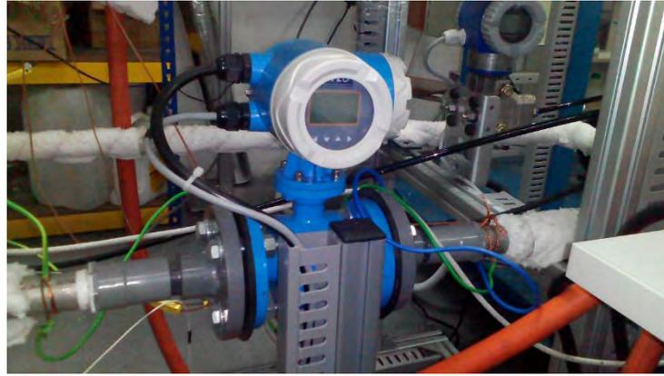
**Figure 3.10:** Photograph of the Electromagnetic flow meter.
