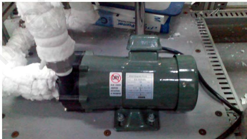
**Figure 3.8:** Photograph of the Magnetic gear pump.
