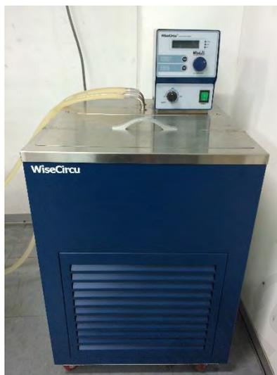
**Figure 3.12:** Photograph of the refrigerated bath circulators.
