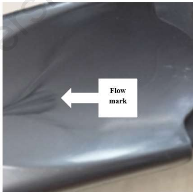
Figure 2.15: Flow mark on the rubber products surface.
