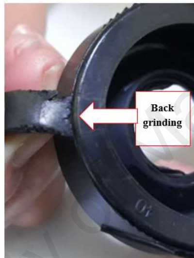
Figure 2.19: Rubber product has back grinding defect.
