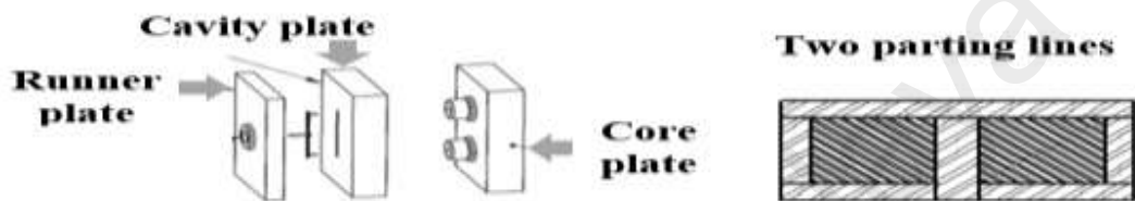
Figure 2.34: Three plate mould. Schematic diagram by Mark T. Maclean-Blevins (2018) and Robinson (2015).
