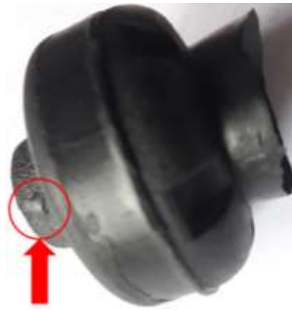
Figure 2.14: Air trapped on the rubber products surface.
