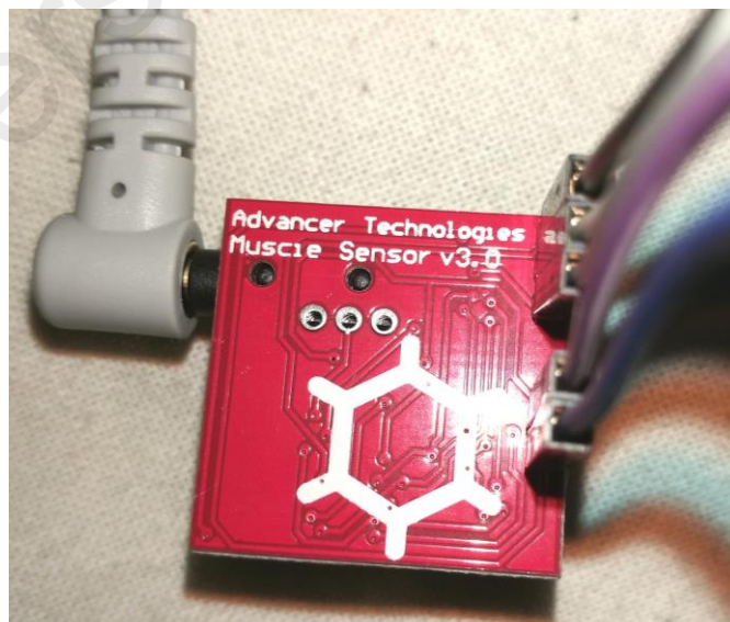
Figure 3.1: EMG sensor board
