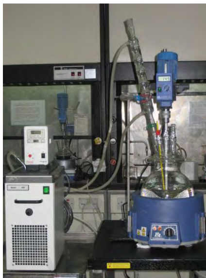
Figure 2.10 : Experimental set-up for etherification of glycerol and tert -butanol in 5 L reactor
