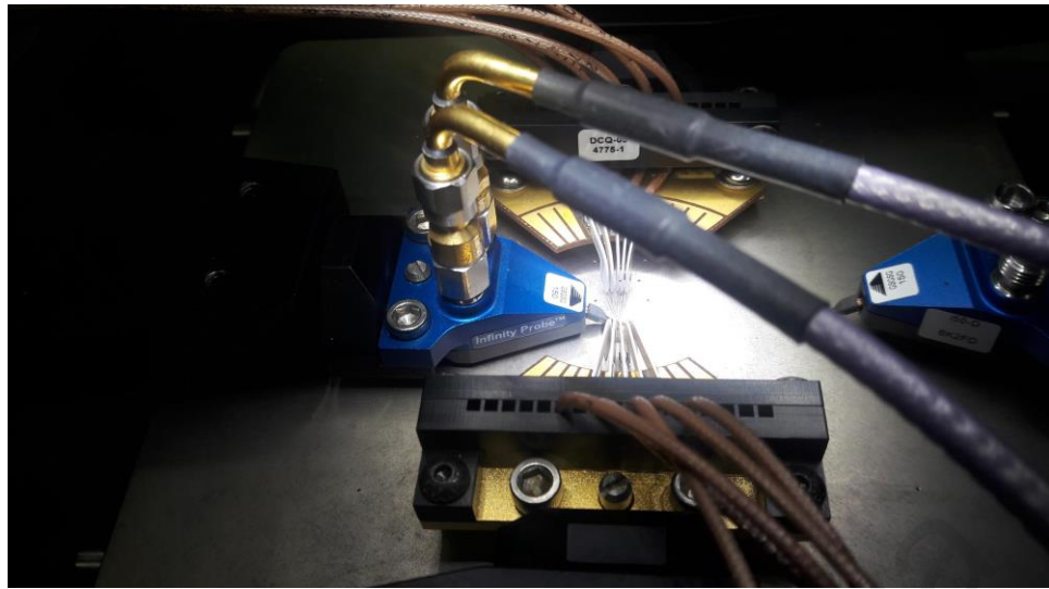
Figure 5.2: Summit 9000 Probe station from Cascade Microtech
