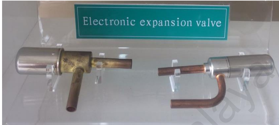
Figure 2.6: Electronic expansion valves (EEVs)
