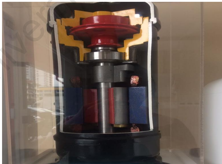
Figure 2.3: Inverter - driven compressor
