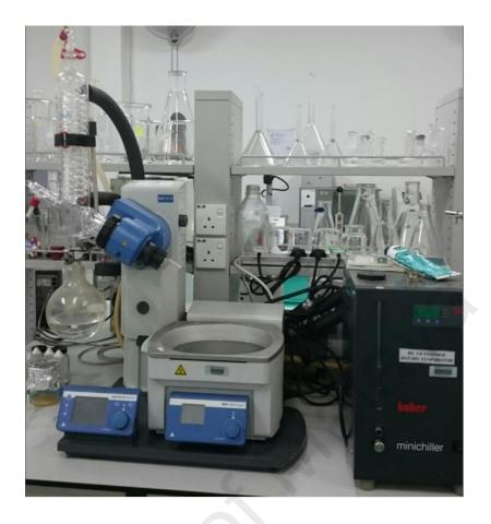
Figure 3.2: Rotary evaporator (IKA RV 10)
