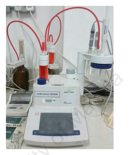
Figure 3.6: Acid value tester from Mettler Toledo
