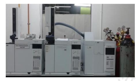
Figure 3.3: Agilent 6890 gas chromatograph
