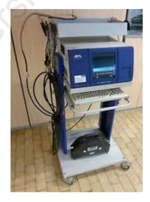
Figure 3.11: AVL Emission tester (series 4000)
