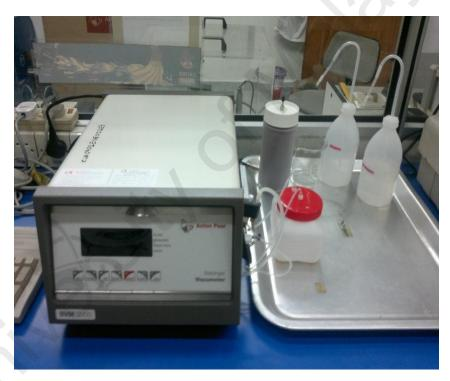
Figure 3.4: SVM 3000 Viscometer
