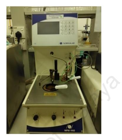
Figure 3.8: NORMALAB NPM 440 flash point tester
