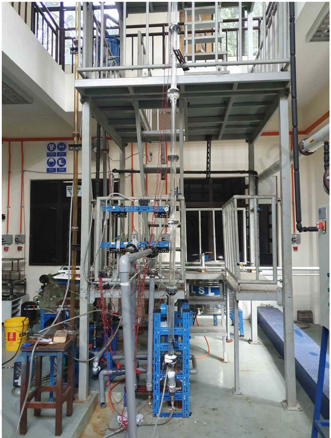
Figure 3.3: Experimental facility of vertical gas-liquid two-phase flow channel at Thermal-Hydraulics Lab, Department of Mechanical Engineering, University of Malaya.
