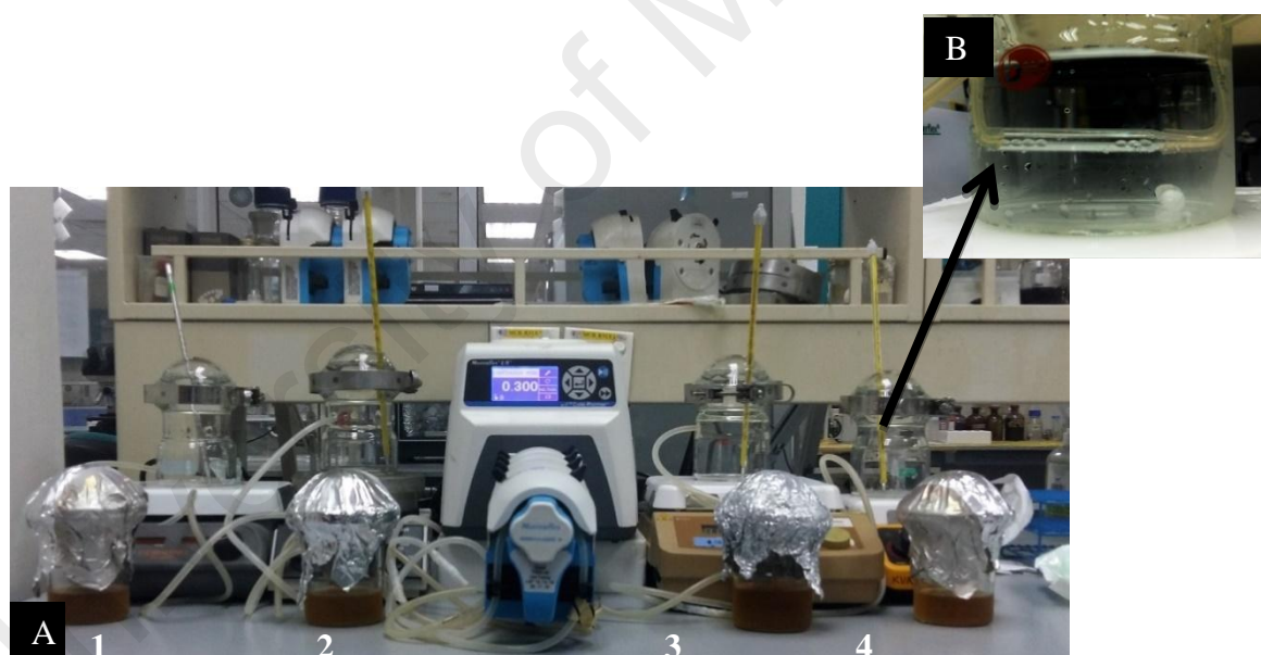
Figure 0.3: A) Four sets of Nordini's Artificial Mouth Model to develop four individual oral biofilms, B) Glass tube containing seven glass beads mimicking oral cavity and teeth respectively.
