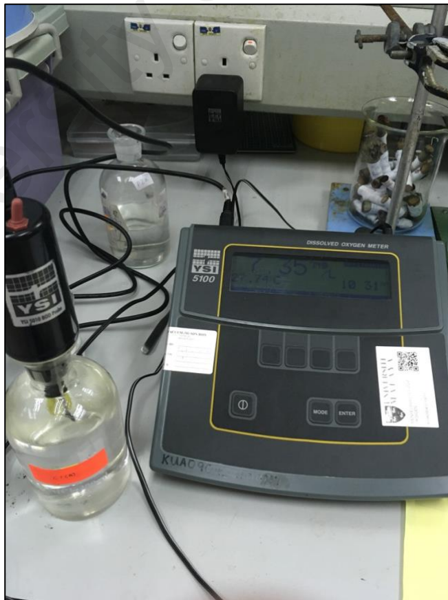
Figure 3.4.1 (b) Dissolve Oxygen Meter to analyze Dissolve Oxygen and Biochemical Oxygen Demand
