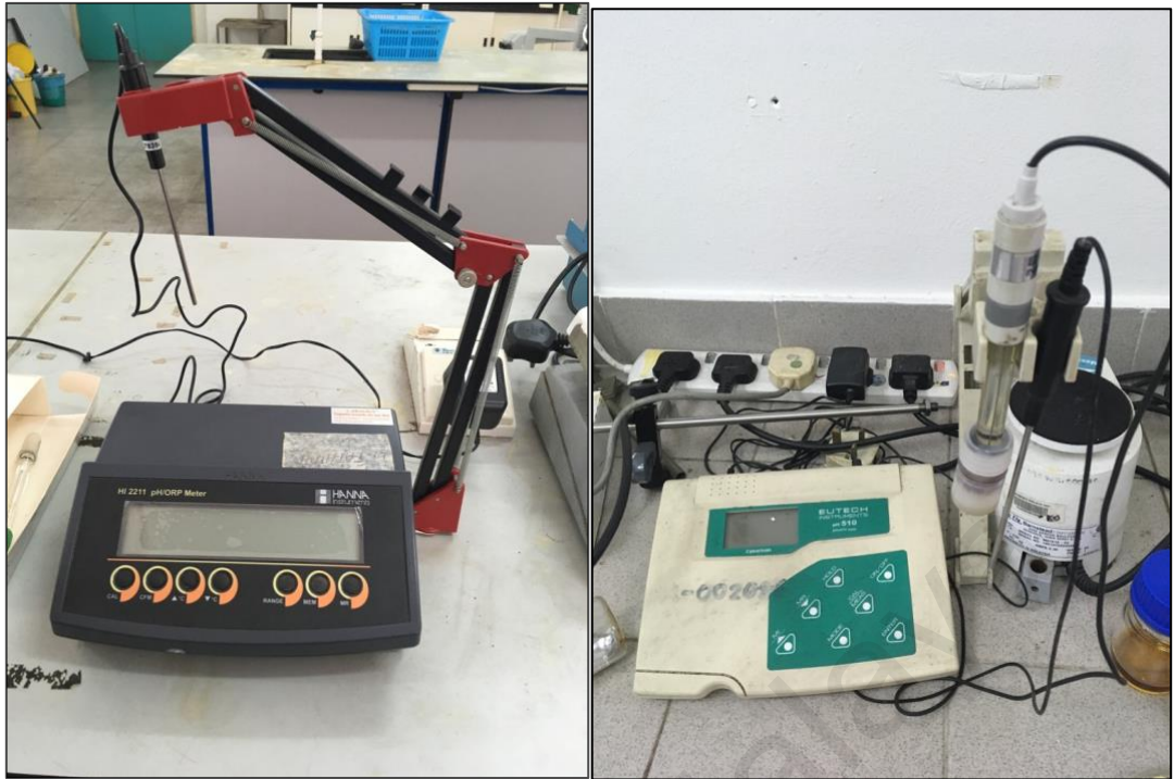
Figure 3.4.1(a) Left side of the picture is pH meter (model Hanna HI 2211) and the right side of the picture is Eutech Instrument pH510. Both instruments are used to detect pH and Temperature of the samples
