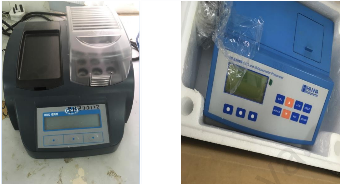
Figure 3.4.1(c) Left side of the picture is HACH DRB 200 and the right side of the picture is Multipara Meter Lab-Photometer. Both equipment is used to analyze COD and Multipara Meter Lab-Photometer to analyze Ammoniacal-Nitrogen
